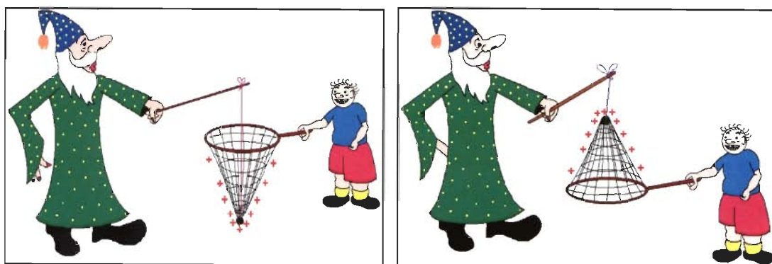
Figure 3.4: Concentration of positive charges (denoted by '+' sign) on the surface of butterfly net, especially at the apex (maximum positive curvature). If the net is inverted by pulling up the thread, charges have the tendency to move towards the new outer surface (Dasgupta, 2005).
