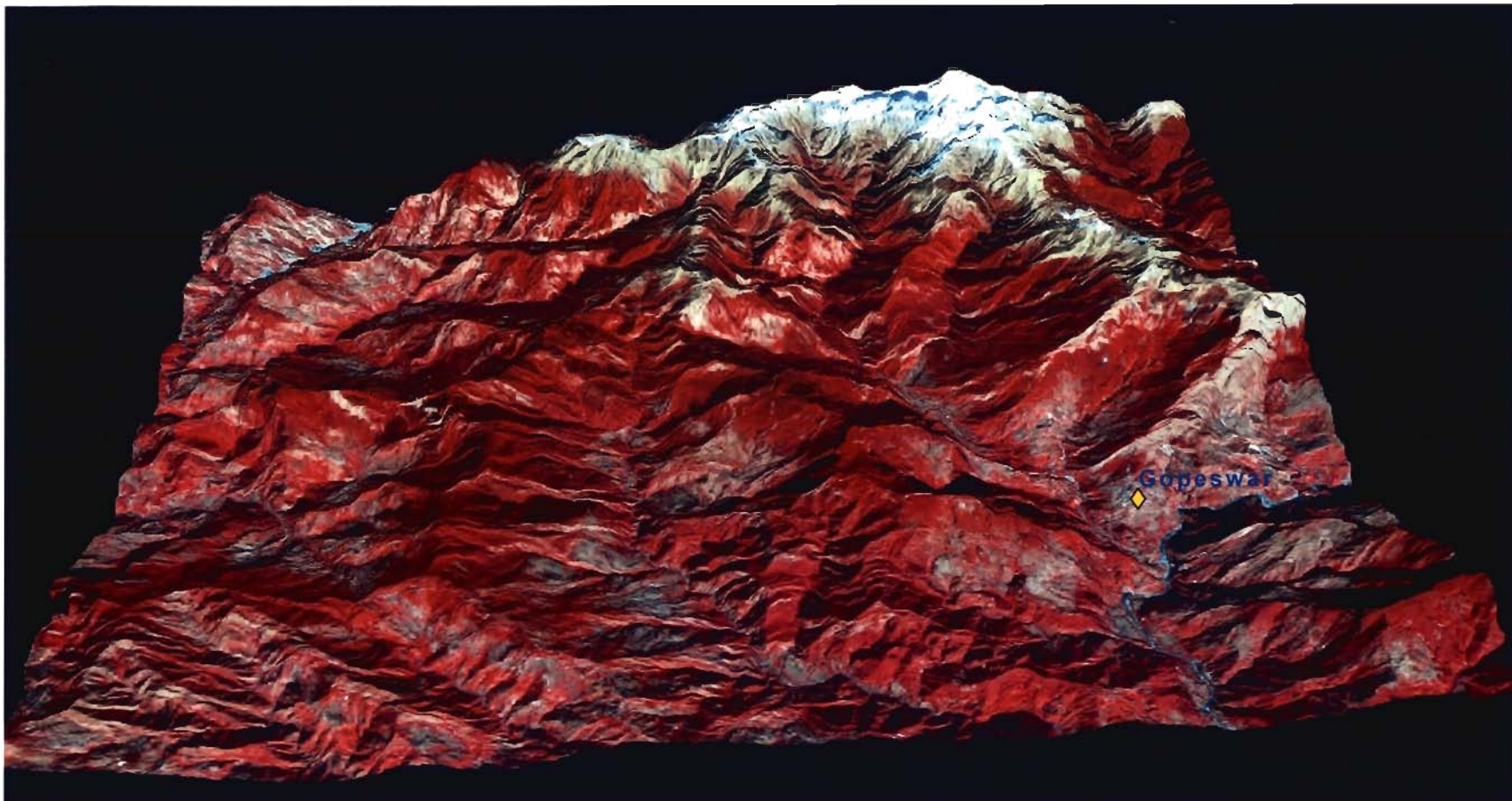
Figure 4.2: IRS-1C LISS-III Colour Infrared Composite in a perspective view (NIR=R, Red=G, Green=B).
