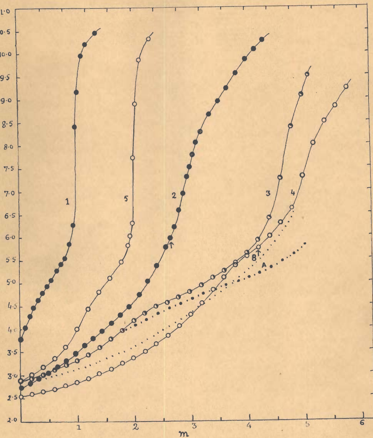
Fig.24. Potentiometric titrations of the normal and mixed ligand chelate systems of oxovanadium(IV) having o-phenanthroline hydrochloride(Phen) and phthalic acid(Ph.A) as ligands: 1,Phen; 2,1:1 VO-Phen; 3,1:1 VO-Ph.A; 4,1:1:1 VO-Phen-Ph.A; 5,Ph.A. A,composite curve of 1 & 3; B,composite curve of 2 & 5. All solutions are 2.5 \times 10^{-3}M in ligand at the start of titration; m = moles of KOH added per mole of the metal ion. Arrows indicate appearance of a solid phase.
