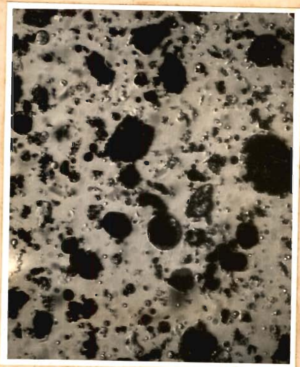
A. Original sample showing angular and rounded opaque grains and spheroids of glass (x 50)
