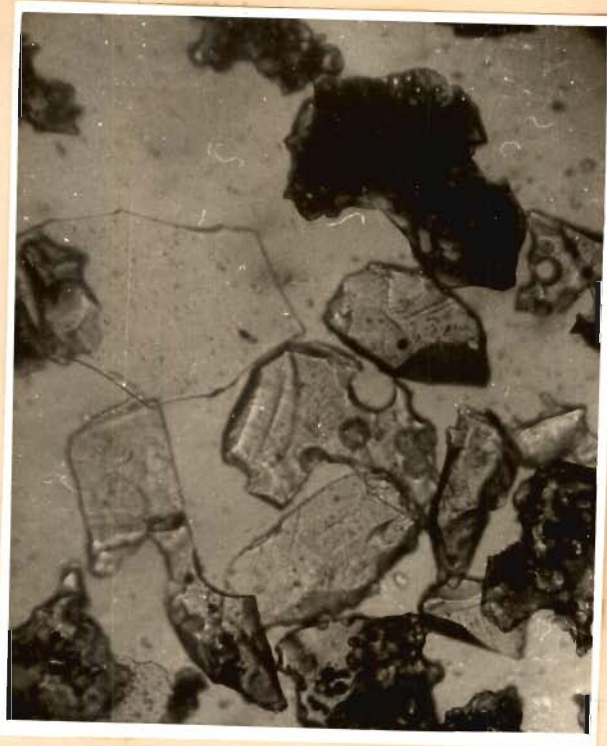
A. Granulated slag-showing subangular to angular grains (x 50)
