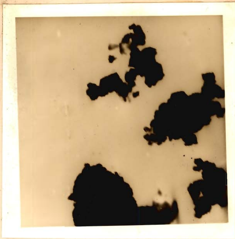
A. Showing fibrous structure with some hexagonal plates of C-A-H (x 17600)
