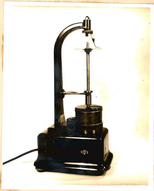
Fig. 15. Showing Mac Michael rotational viscometer; the spindle-plunger assembly is suspended by a wire and dips into the rotatable cup.
