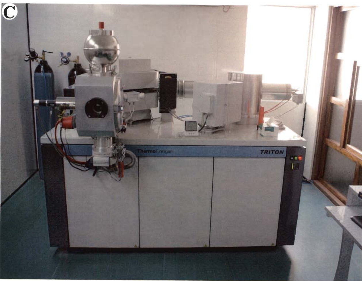
Figure 3.3. Instruments used at National Facility of Geochronology/ Isotope geology Laboratory at the Institute Instrumentation Centre, IIT Roorkee. A. Ion Exchange Column. B. Sample Evaporation Unit. C. Thermal Ionization Mass Spectrometer (TIMS)-Triton T1 Model.
