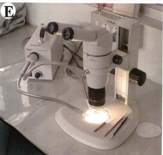
Figure 3.2. Instruments used during sample preparation for Rb-Sr analysis at Sample Preparation Laboratory, Department of Earth Sciences, IIT Roorkee. A. Jaw Crusher. B. Ball Mill. C. Mica Vibrator. D. Isodynamic Separator. E. Binocular Microscope
