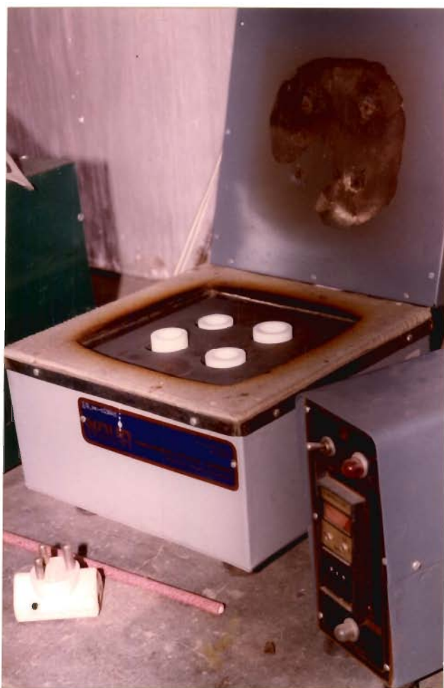
Figure 4.5 Etching bath with temperature controller, used in the present study to etch zircon mounts
