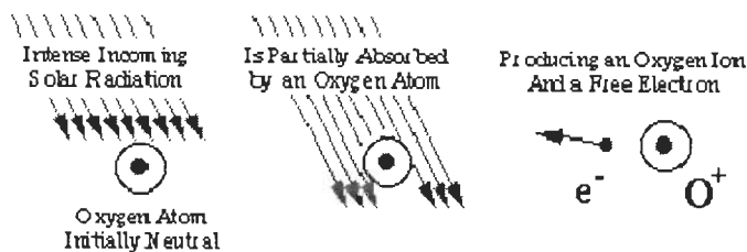
Figure 1.1 Production of electron and ion due to solar radiation.
