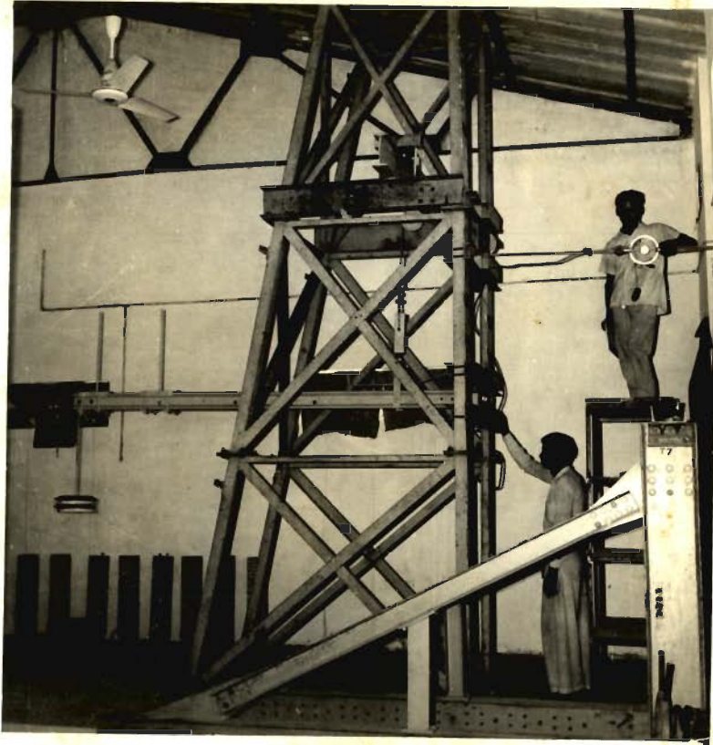
FIG.43- 5-Tonne Reaction Frame With Loading Beam and Weights and Proving Ring
