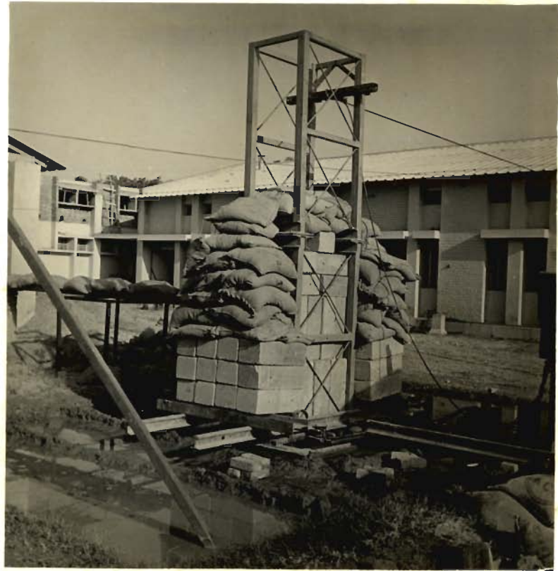
FIG.44- Field Well In-situ With Loading Frame, Loading Blocks, Datum Beams and Loading Cable
