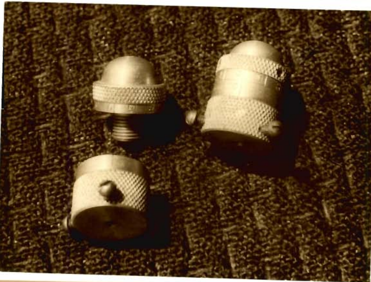
P 7: MICROMETER TENSIONING CUM GRIPPING DEVICE
