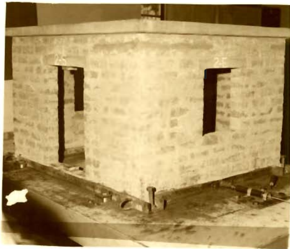
PHOTO 4.2 - SLIDING TYPE, 1/4 SCALE, MODEL NO. 2 WITH BASE FREE TO SLIDE
