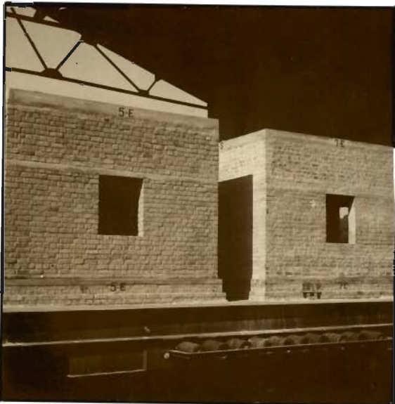
PHOTO 5.7 _ MODELS 5 AND 7 (SLIDING TYPE IN MUD AND CEMENT MORTAR) BEFORE SHOCK LOADS
