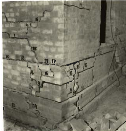
PHOTO 5-67-SEVERE DAMAGE OF NORTH-EAST AND NORTH-WEST CORNERS (MODEL 4)
