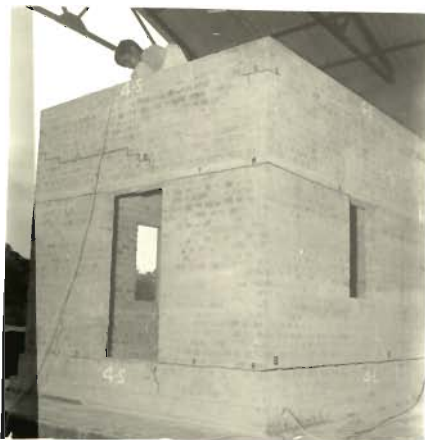
PHOTO 5.48_ HORIZONTAL CRACKS IN SOUTH AND EAST WALLS (MODEL 4)
