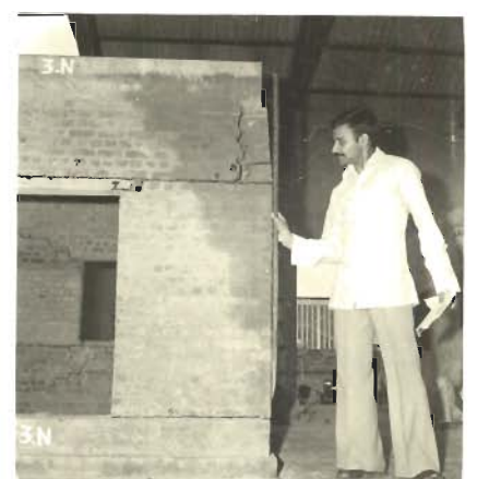
PHOTO 5.44 _ WEST PIER OF NORTH WALL SLID OUTWARD ( MODEL 3 )
