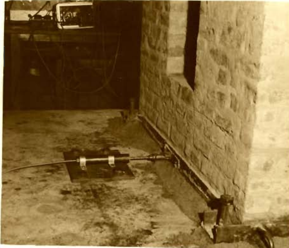
PHOTO 4.1 - SLIDING TYPE, 1/4 SCALE, MODEL NO. 1 WITH BASE FREE TO SLIDE
