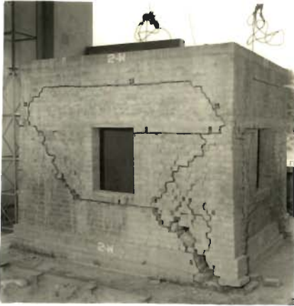
PHOTO 5.27_ BIG GAP AT BOTTOM OF SOUTH-EAST AND SOUTH-WEST CORNERS ( MODEL 2 )
