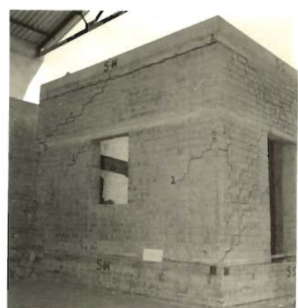
PHOTO 5.80 FEW HORIZONTAL AND DIAGONAL CRACKS IN WEST WALL (MODEL 5)
