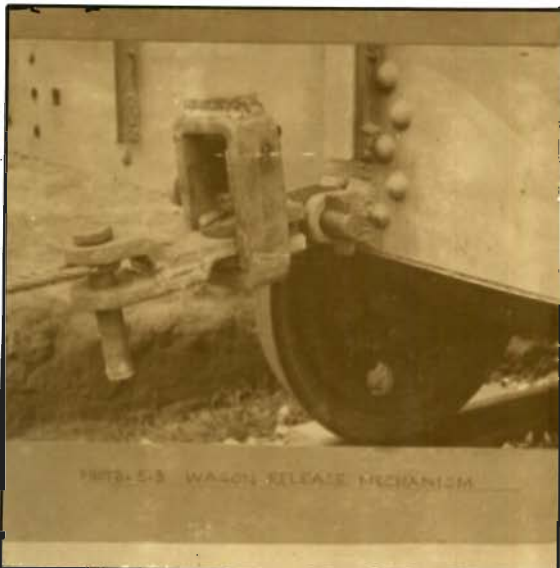
PHOTO 5.3 - WAGON RELEASE MECHANISM
