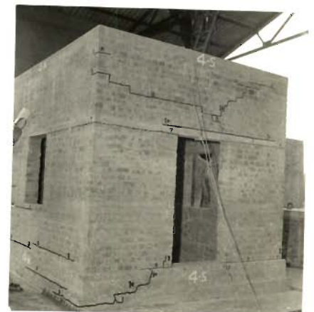
PHOTO 5.52_ DIAGONAL AND HORIZONTAL CRACKS IN SOUTH WALL (MODEL 4)
