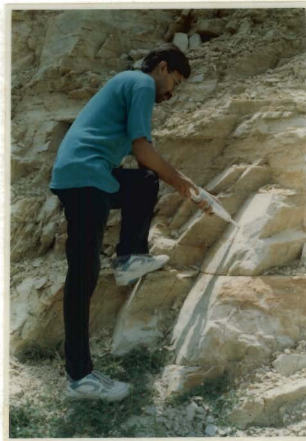
Plate 5.4 Use of Schmidt hammer on joint planes
