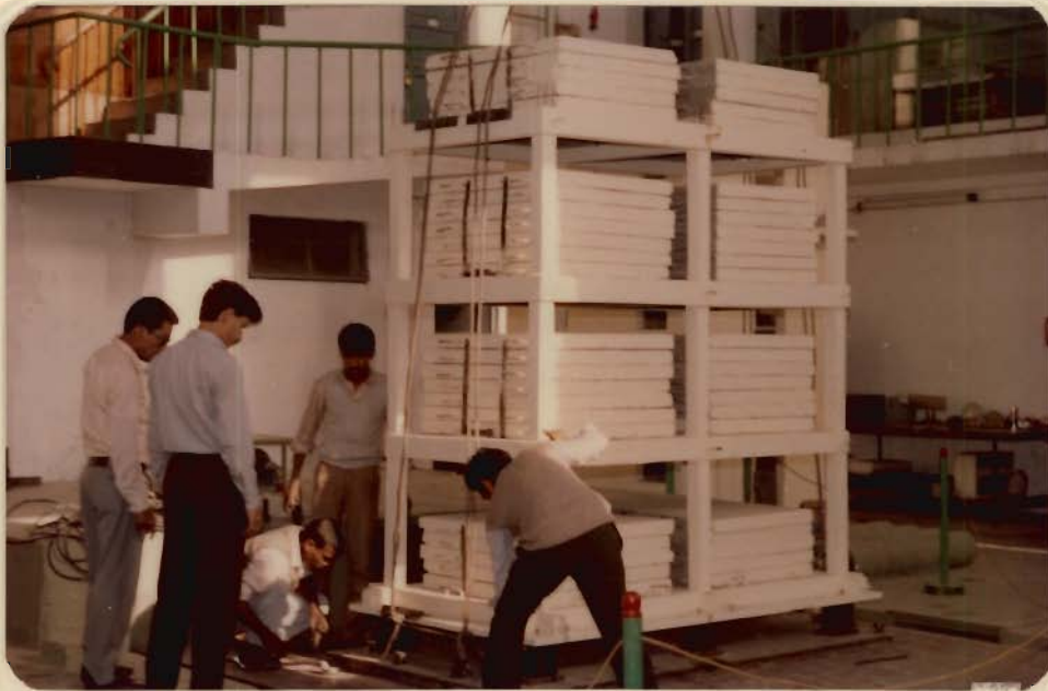
Photo 4.3 : Placing of the Test Structure on the Shake Table
