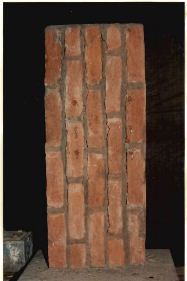
Fig.3.9 Failure of Brick Masonry Piers subjected uniaxial Loading
