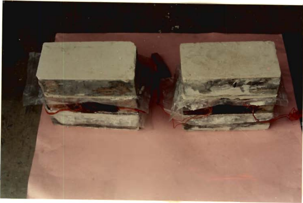
(a) Brick Specimen Placed in a Three Brick High Brick Prism
