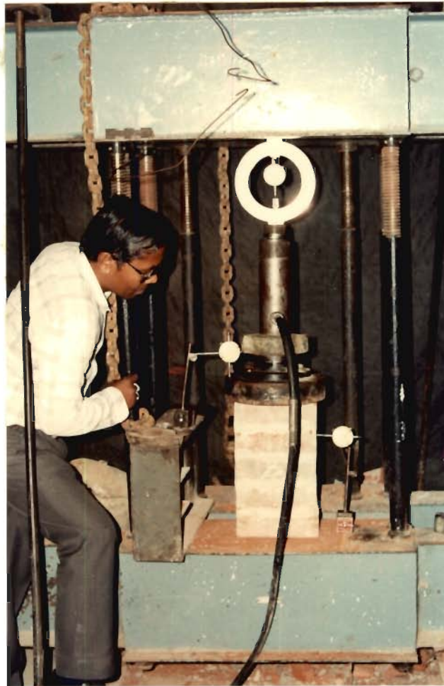
(a) Setup for Compression Test for Masonry Prism
