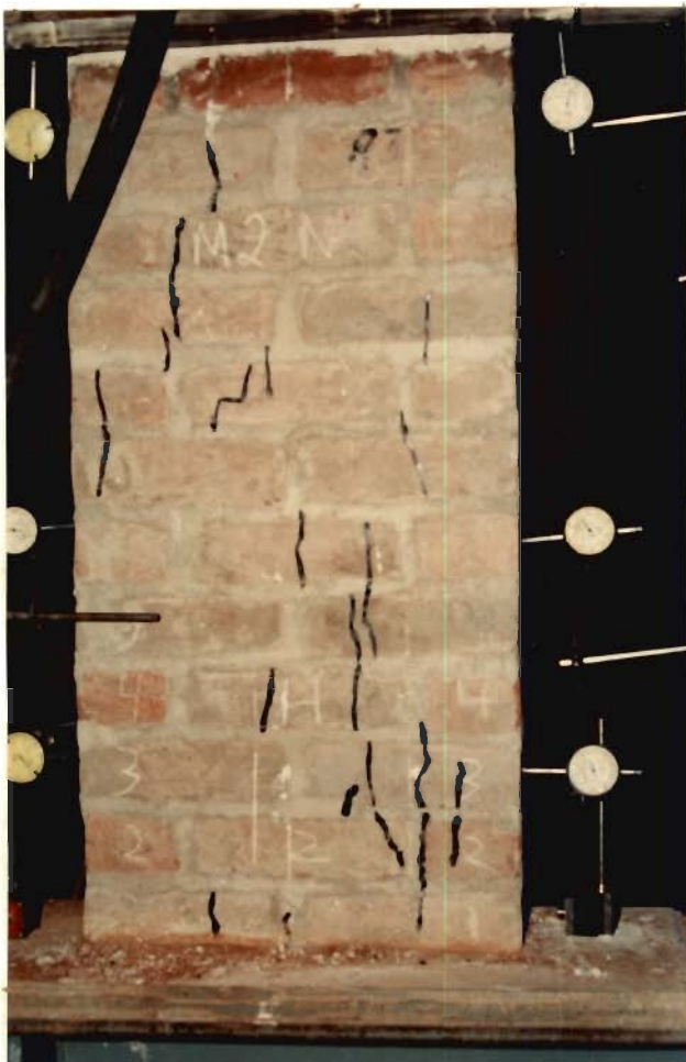
Fig.3.9 Failure of Brick Masonry Piers subjected uniaxial Loading
