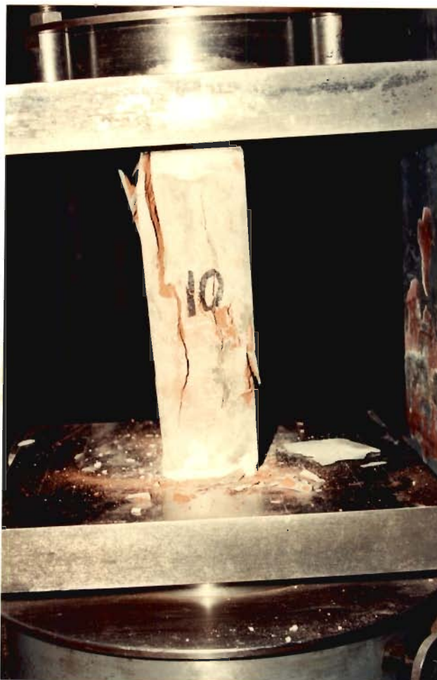
(b) Typical Splitting Failure of Brick
