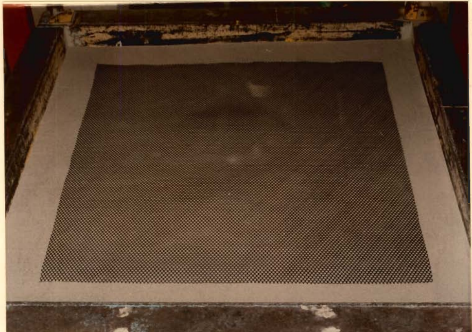
FIG. 3.12 LAYING OF REINFORCEMENT LAYER IN SAND BED
