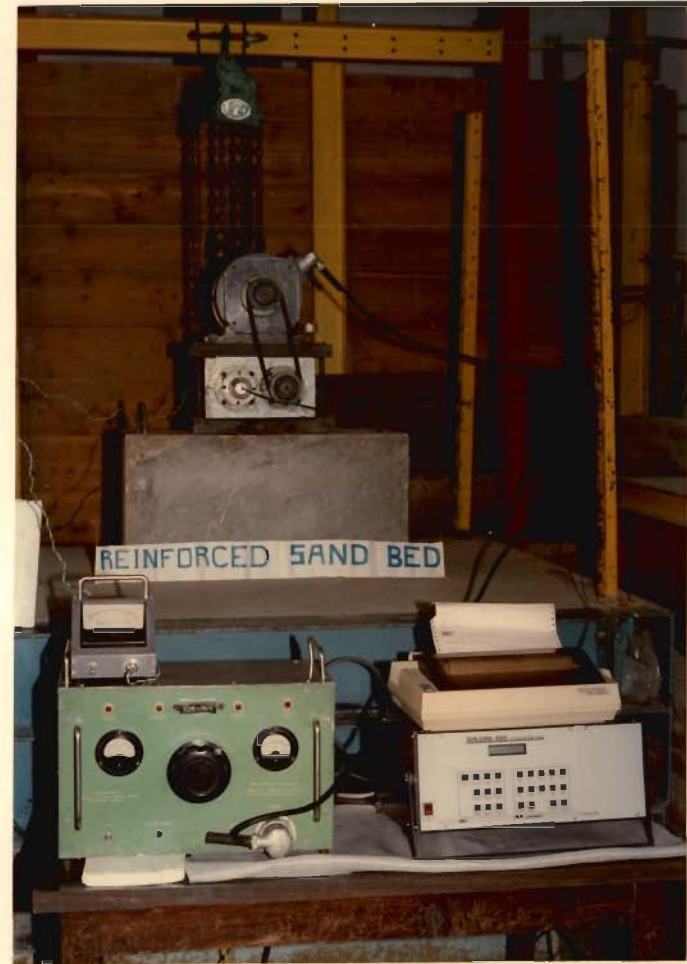
FIG. 3-16 SOIL DATA LOGGER-4201
