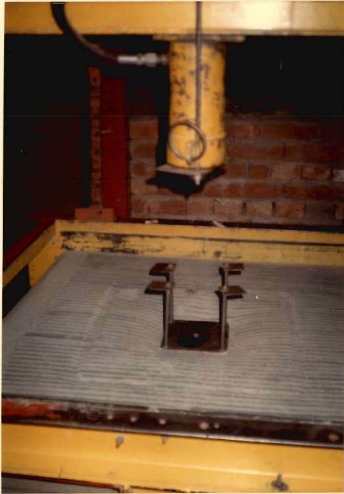
FIG. 3.8 SETTLEMENT PATTERN IN CYCLIC PLATE LOAD TEST ON GEOGRID REINFORCED SAND BED
