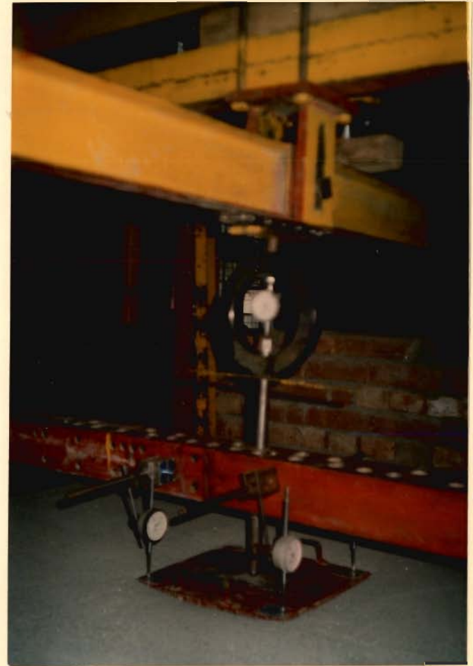
FIG. 3.9 CYCLIC PLATE LOAD TEST IN PROGRESS
