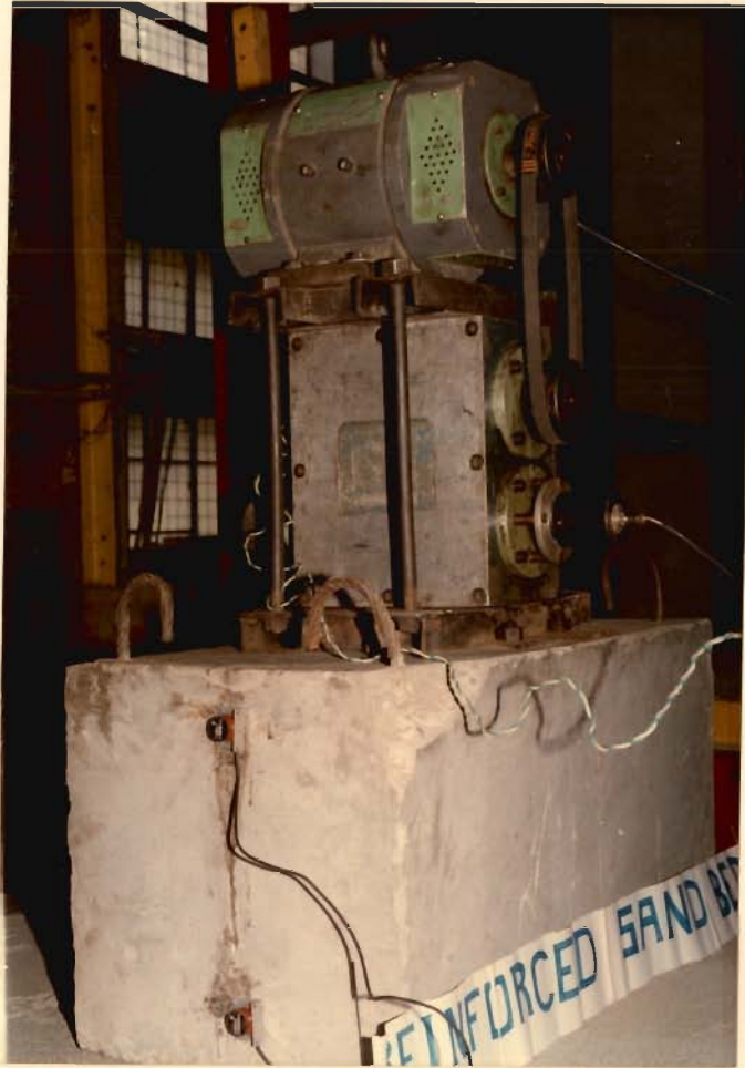
FIG. 3-15 EXPERIMENTAL SET-UP FOR HORIZONTAL BLOCK VIBRATION TESTS
