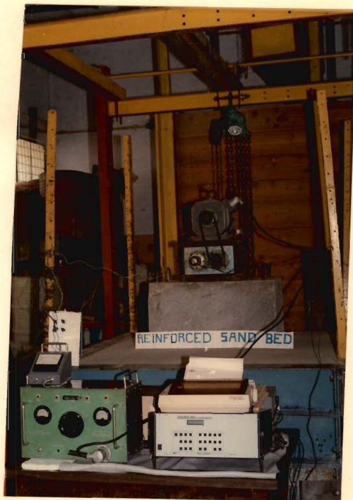
FIG. 3.13 EXPERIMENTAL SET-UP FOR VERTICAL BLOCK VIBRATION TEST
