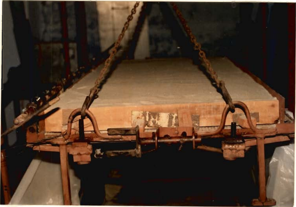
FIG.3.2.5 SUSPENDED SRA FILLED WITH SAND.
