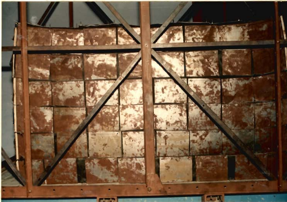
FIG. 4.4.14 A VIEW OF THE RE-TEST EMBANKMENT AFTER THE DYNAMIC TESTS IS COMPLETED.
