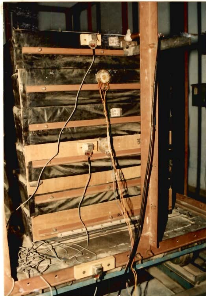
FIG. 4. 4. 12 VIEW OF THE LONGITUDINAL FACE OF THE EMBANKMENT WITH ACCELERATION PICKUPS IN POSITION.
