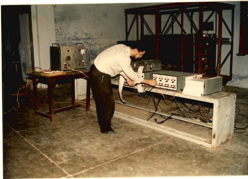
FIG. 4.4.13 A VIEW OF THE FREE STANDING RE TEST EMBANKMENT ON SHAKE TABLE AND THE AMPLIFIERS AND RECORDERS JUST BEFORE THE DYNAMIC TESTING.
