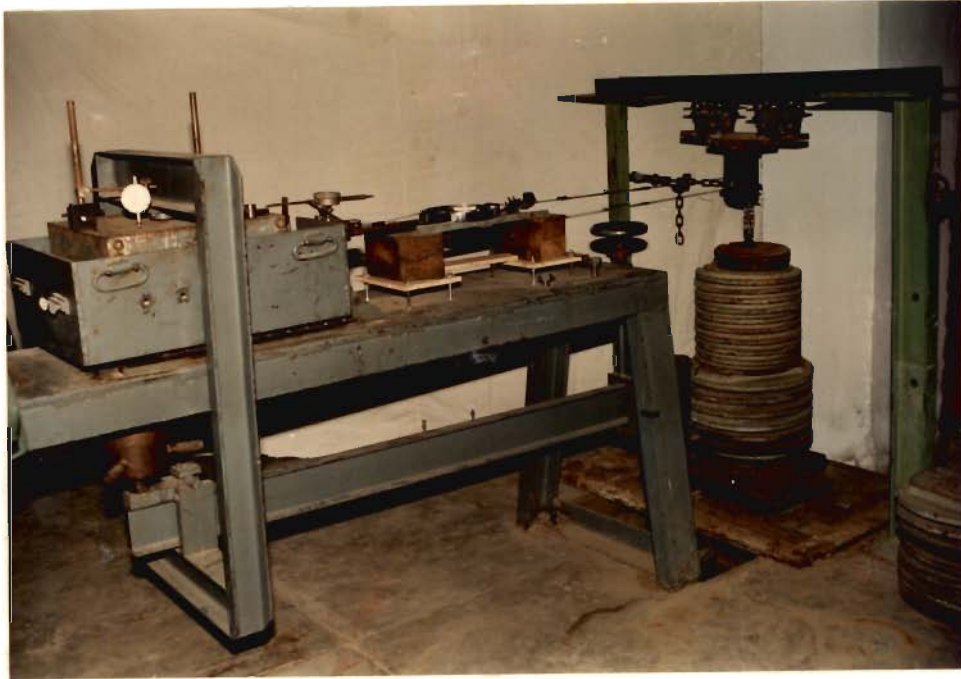
FIG. 4.3.7 TEST SETUP FOR PULLOUT RESISTANCE WITH WEIGHTS PLACED ON THE LOADING HANGER.
