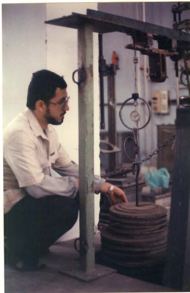
FIG. 4.3.3 CALIBRATION SETUP FOR PROVING RING.
