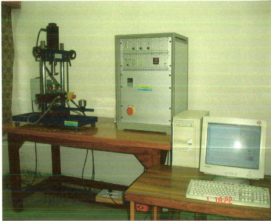
Fig. 3.13: Photographic views of the tribological testing machine (MTM 60)
