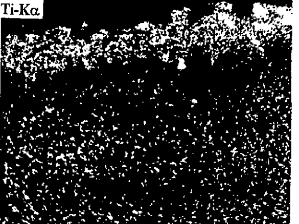
Fig. 5.21: BSEI and X-ray mapping of the cross section of alloy C (Superni 75) after cyclic hot corrosion at 900 o C in Na 2 SO 4 -60%V 2 O 5 + MgO. (X 600)
