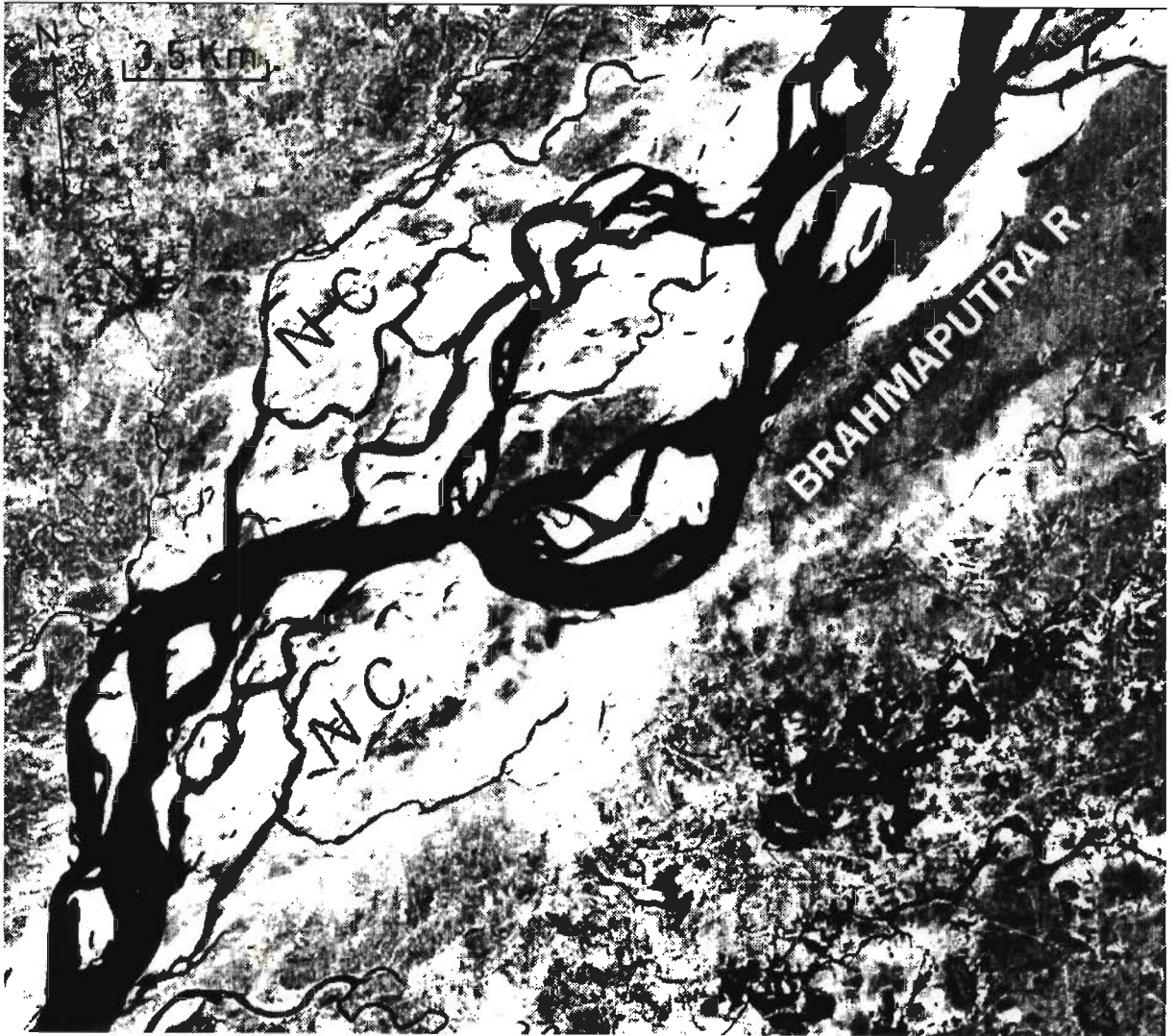
Fig. 5.21 Digitally enhanced image (IRS: LISS-II, Band-4) showing development of new channels on the north and south bank of the river. NC-New Channel.
