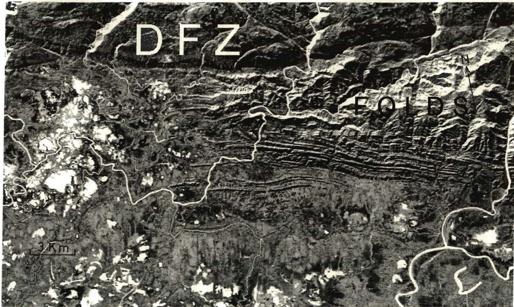
Fig. 5.10 Digitally enhanced image (IRS: LISS-II, Band-4) showing the E-W trending folds in soft sediments south of the Dauki fault zone (DFZ). This is an inverse image.
