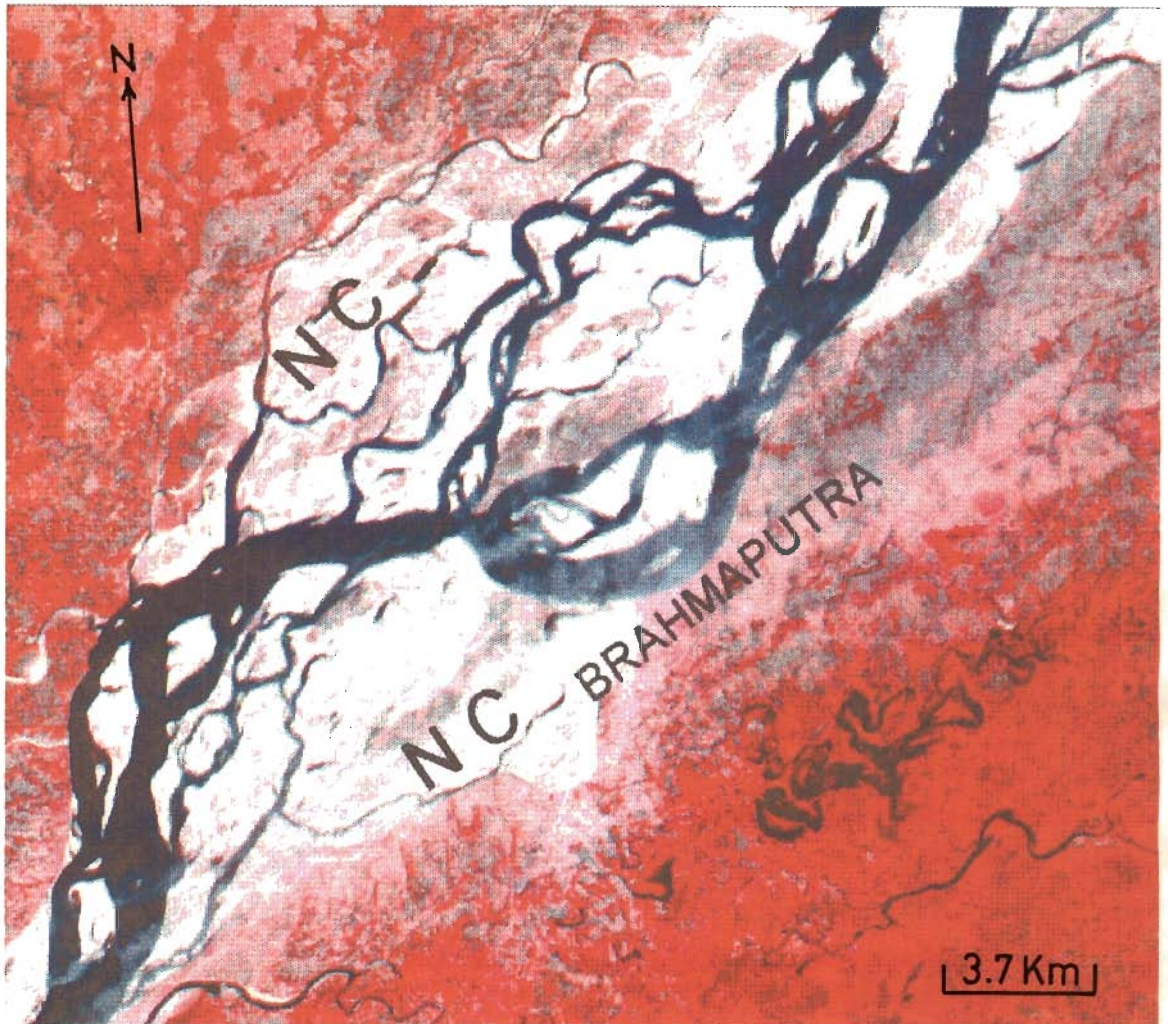
Fig. 5.23 Enhanced colour composite (IRS: LISS-II) image showing development of new channels on the north and south bank of the river. NC - New Channel.
