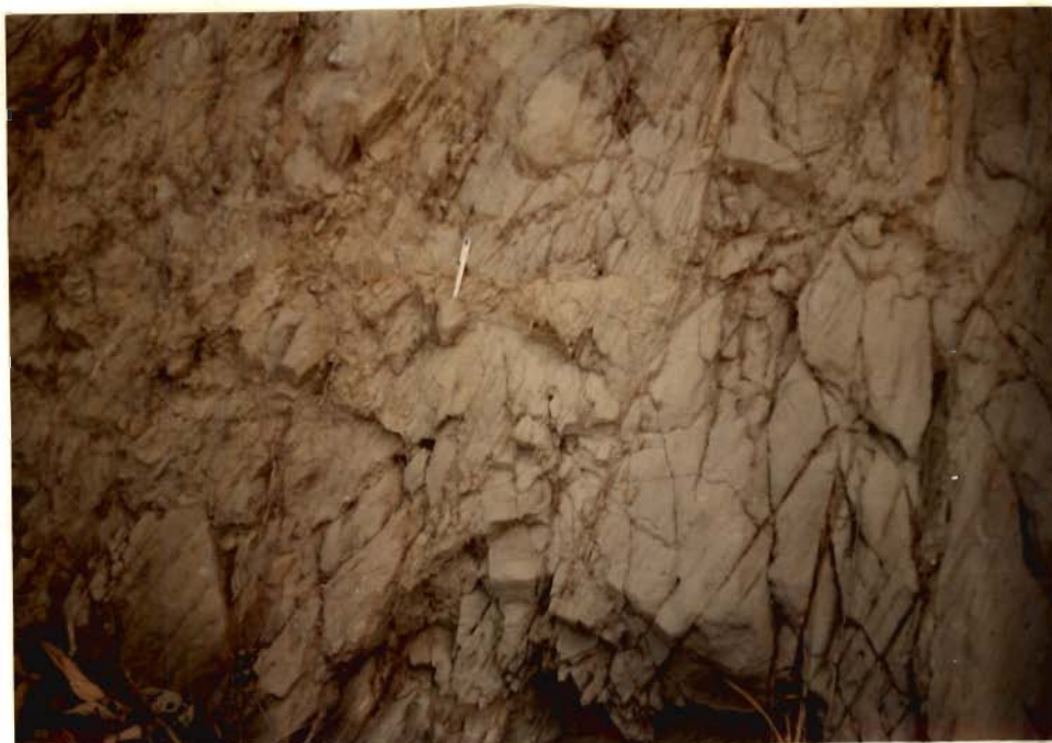
Figure 4.17 (A). Field photograph showing multiple fractures in shale. Loc.- 10 km west of Balat.
