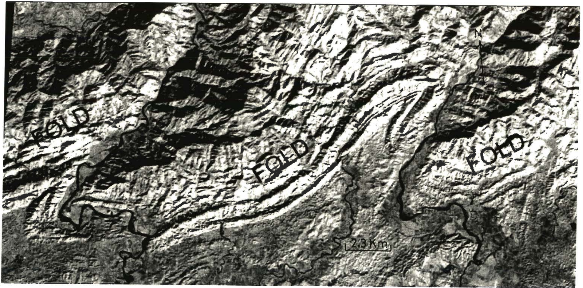
Fig. 5.12 Digitally enhanced image (IRS: LISS-II, Band-4) showing the NE-SW trending sedimentary folds with curved limbs and compressed noses which are displayed in the area south of the Haflong thrust zone (HTZ).
