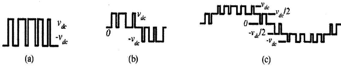
Fig. 3.5 Pulse width modulation pattern: (a) two-level scheme with bipolar; (b) two-level Scheme with unipolar; (c) three-level scheme.
