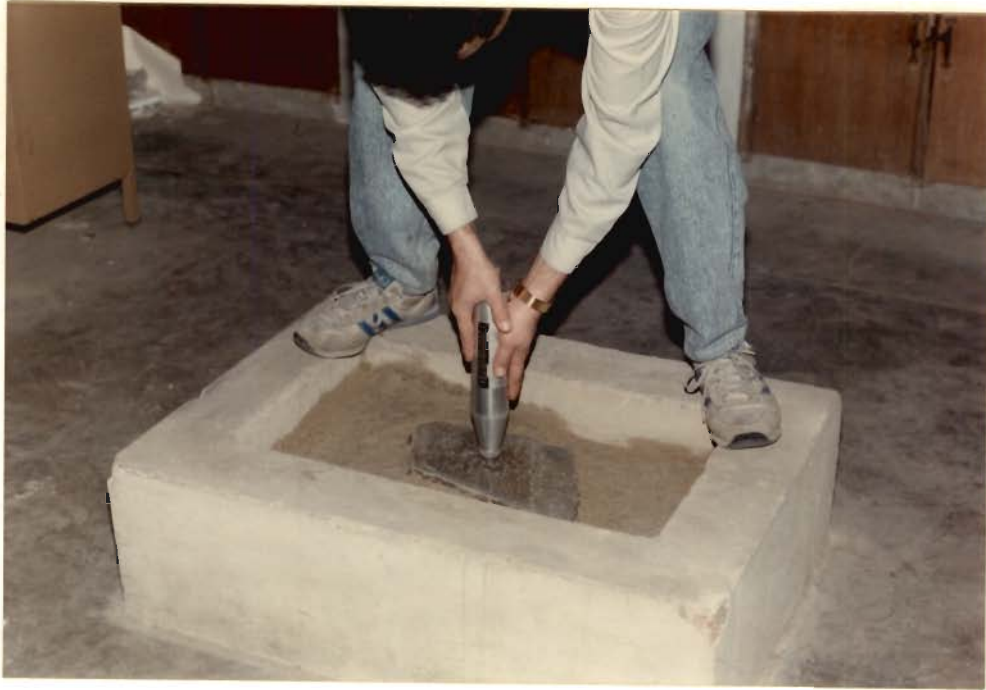
Fig. 5.16 : Measurement of Uniaxial Compression Strength (JCS) by L-type Rebound Hammer
