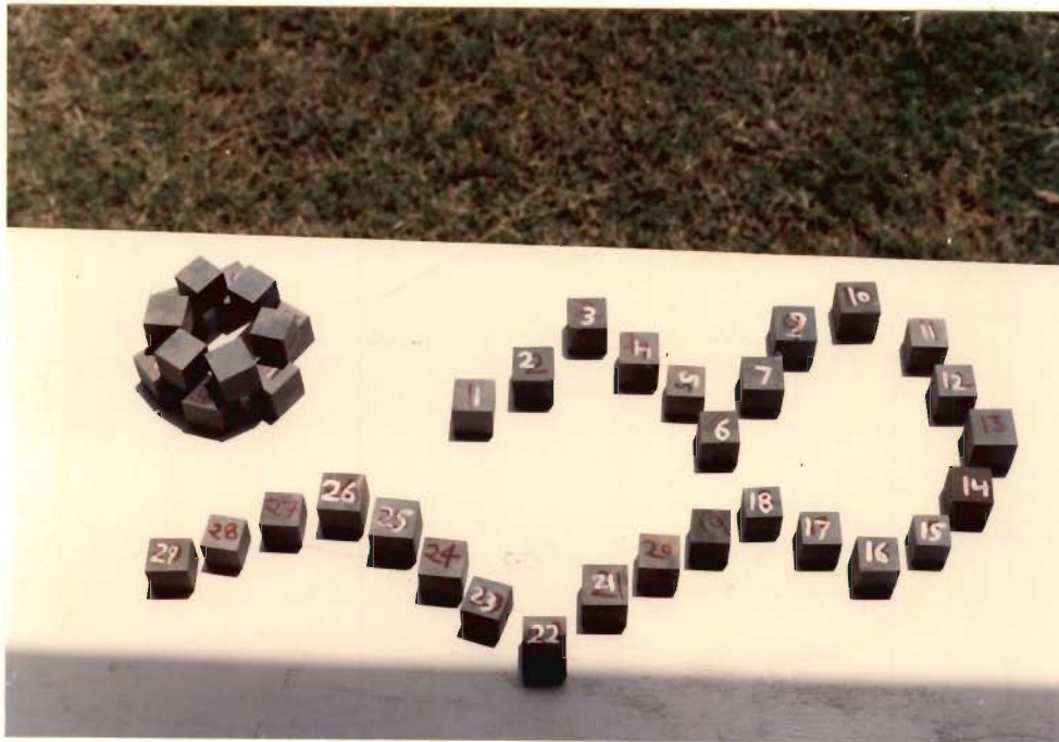
Fig. 5.17 : Rock Cubes Preparation for Measurement of Uniaxial Compressive Strength (JCS)
