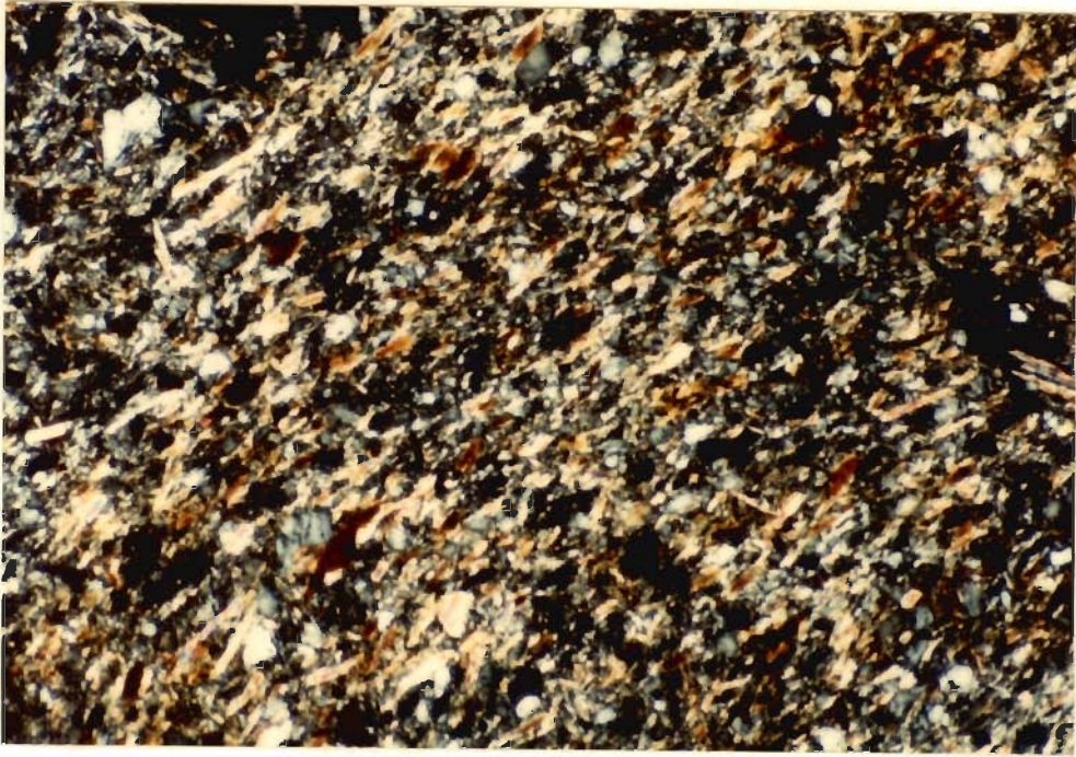
Fig. 4.39 Strongly oriented parallel striated b-fabric in C horizon of the Lower Kosi-Gola Plain, Pedon PA7, XPL, Frame length 1.4 mm.
