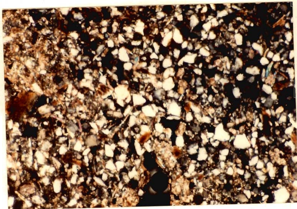
Fig. 4.11 Moderately well sorted coarse fraction showing monic and geric related distribution. Pedon B14, C horizon Rapti Floodplain, Frame length 1.4 mm, XPL.
