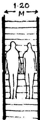
FIG. 5.6.2 MIN. WIDTH OF STAIRCASE FLIGHT FOR COMFORTABLE CIRCULATION
