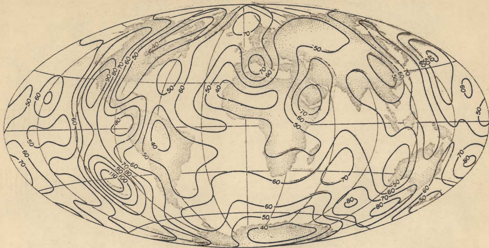
Degree 12 spherical harmonic representation of global heat flow using observations supplemented by predicted heat flow where no observations exist. Heat flow in \text{mW m}^{-2} .
