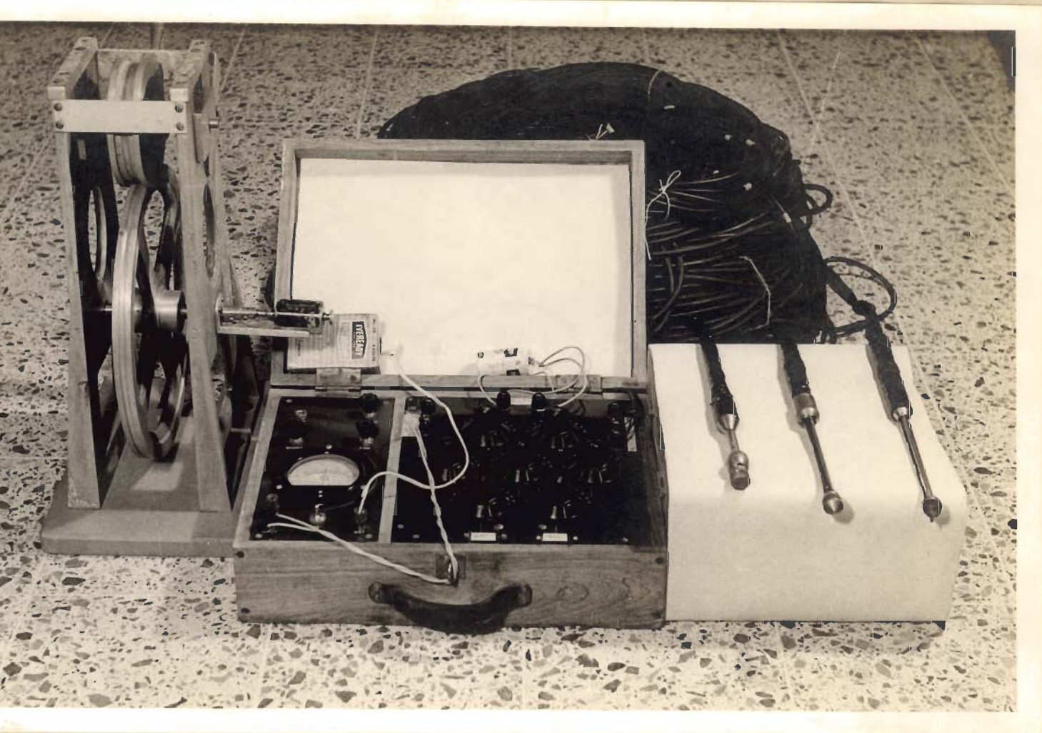
FIG. II-1 Equipment for measurement of Geothermal Gradients, showing thermistor probes, cable, Pully system and the bridge.
