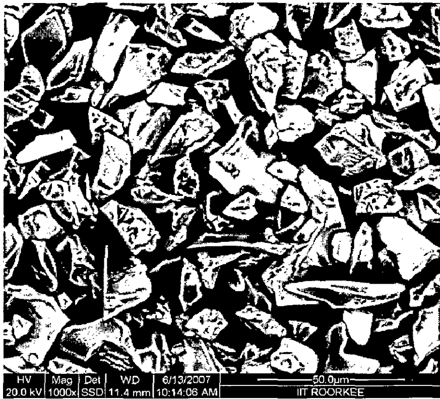
Fig. 4.2: Scanning electron micrographs showing morphology of \text{Al}_2\text{O}_3 -3wt% \text{TiO}_2 powder.
