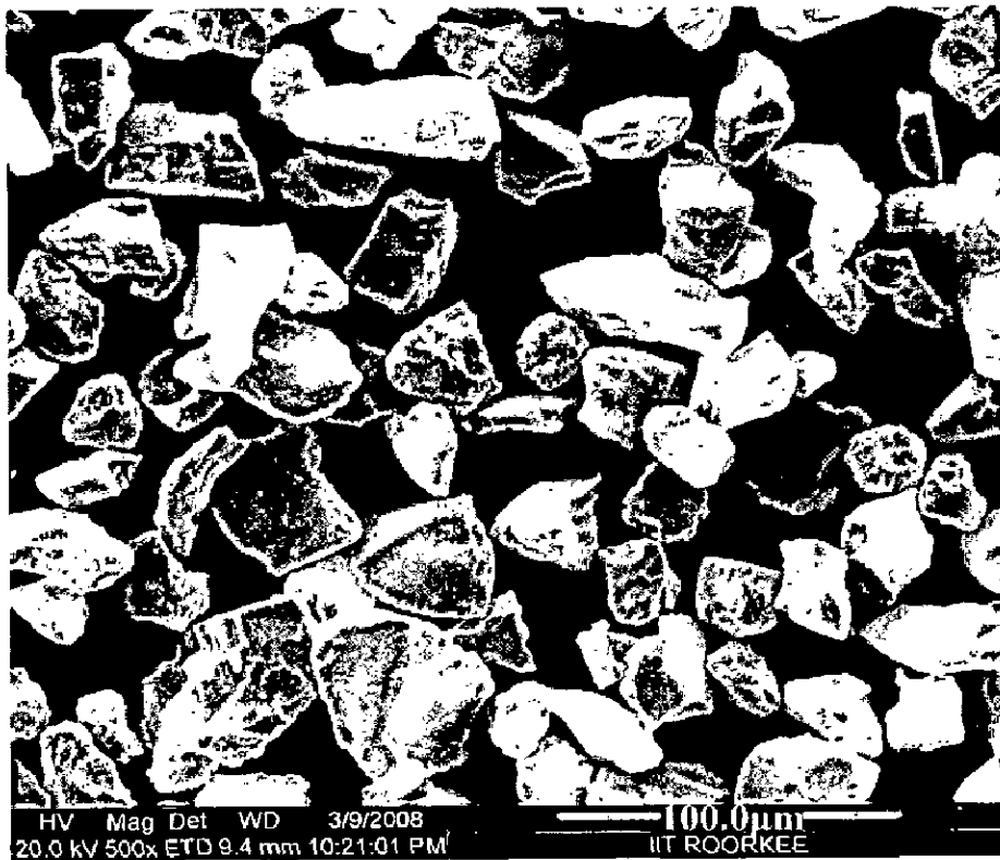
Fig. 3.7: Scanning electron micrograph of the Alumina Erodent particles.
