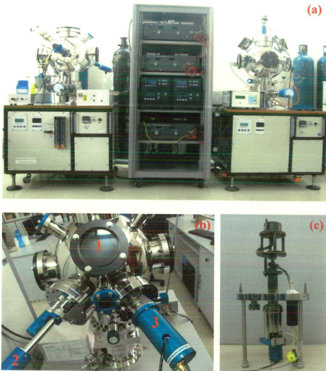
Figure 2.2 (a) Magnetron sputtering system, (b) Back view of sputtering system exhibit position of sputtering guns and (c) Substrate heater (Range: RT-850 °C).
