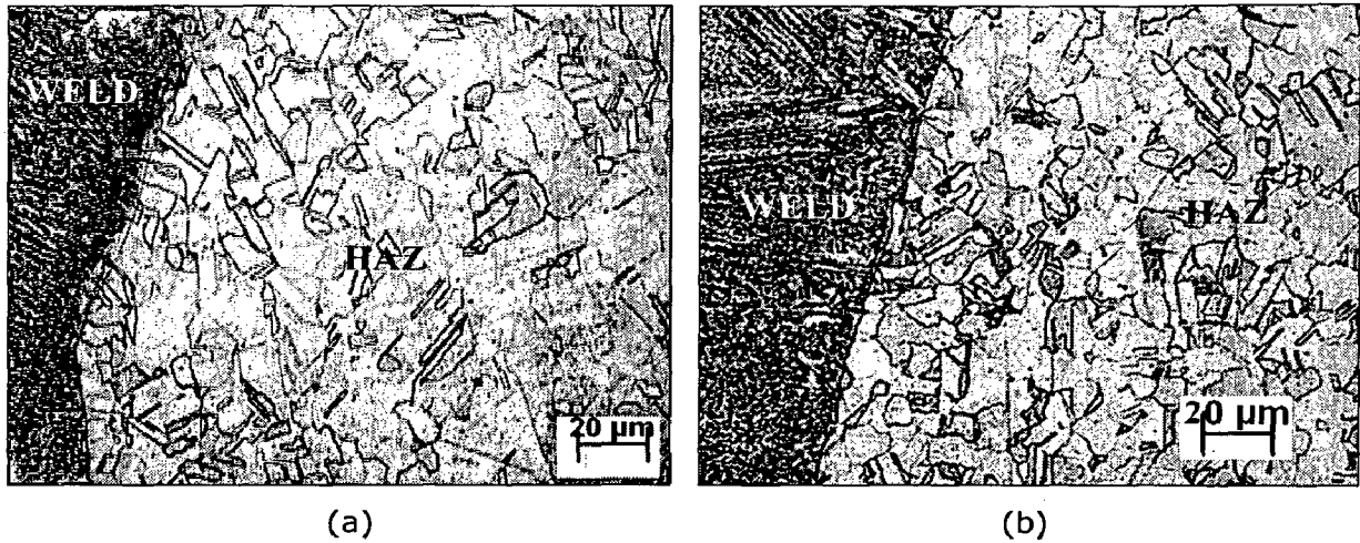
Fig. 5.66 Typical microstructures observed in heat affected zone adjacent to fusion line of narrow groove SMA welds at a weld width of (a) 14mm and (b) 11mm.
