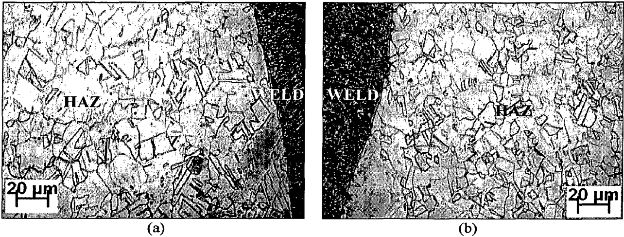
Fig. 5.42: At a given \Omega of 7.7 \pm 0.5 kJ/cm typical microstructure of heat affected zone adjacent to fusion line of P-GMA weld joints at different \phi of (a) 0.05 and (b) 0.25.
