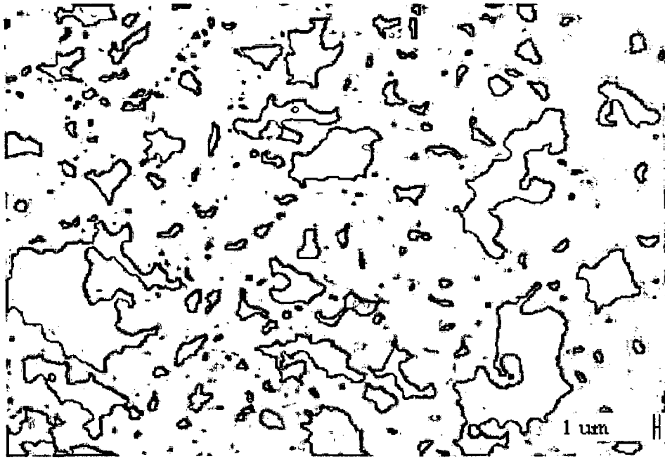
Fig. 5.53 Image analysis for calculating volume fraction of SiC particles in SiC p reinforced MoSi 2 matrix after processing at high temperature.
