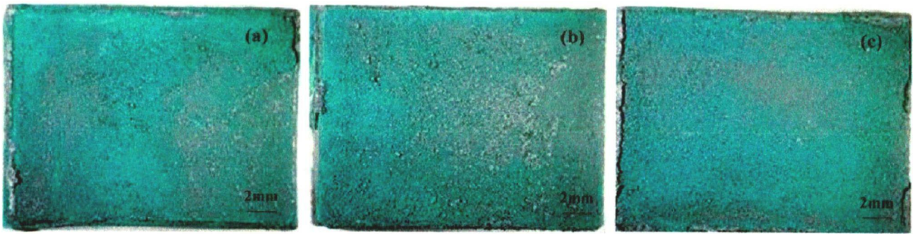
Fig. 6.21 Surface macrograph of NiCoCrAlYTa coated superalloys subjected to hot corrosion in \text{Na}_2\text{SO}_4\text{-60\%V}_2\text{O}_5 environment at 900^\circ\text{C} for 100 cycles, (a) superni 75, (b) superni 718, (c) superfer 800H.
