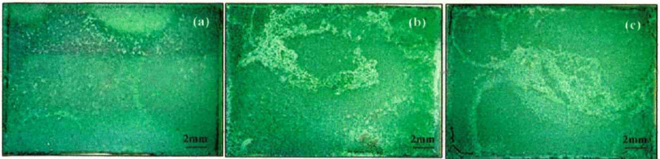
Fig. 5.32 Surface macrograph of NiCrAlY+0.4wt%CeO 2 coated superalloys subjected to cyclic oxidation in Na 2 SO 4 -25%K 2 SO 4 environment at 900 °C for 100 cycles, (a) superni 75, (b) superni 718 and (c) superfer 800H
