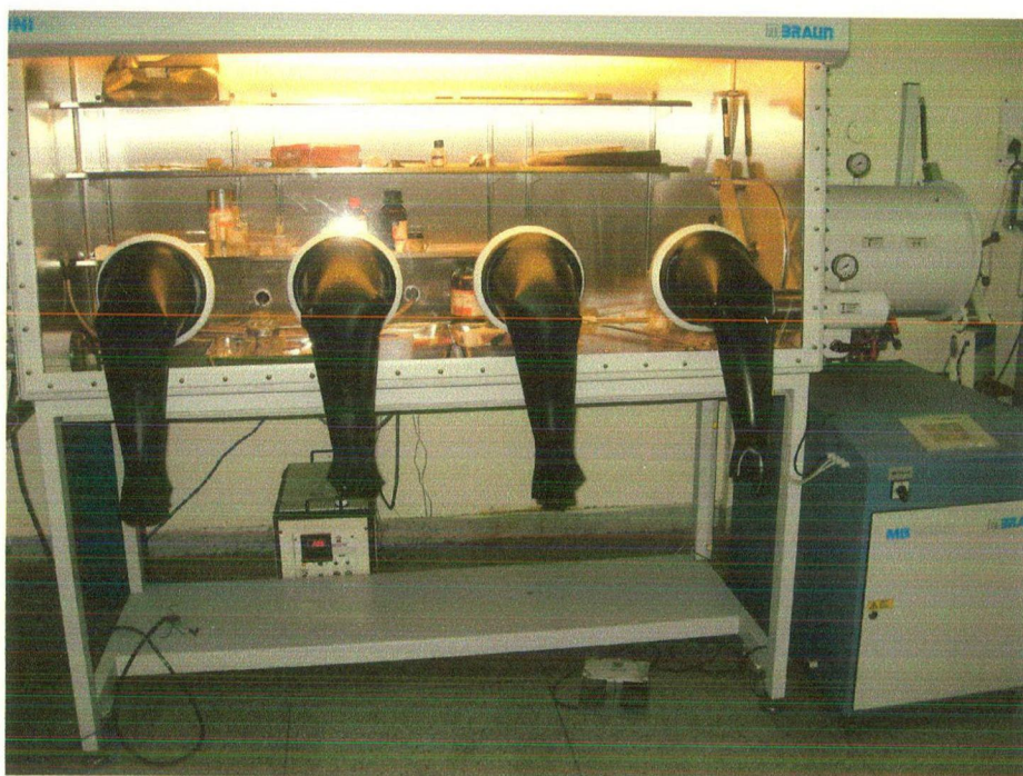
Fig. 3.6: Glove Box (MBRAUN) maintained at < 0.1 ppm of oxygen and moisture
