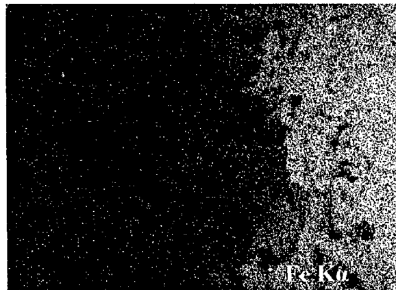
Fig.6.17 BSEI and elemental X-ray mapping along the cross-section of the NiCrAl coated T22 steels subjected to hot corrosion for 50 cycles in \text{Na}_2\text{SO}_4 -60% \text{V}_2\text{O}_5 environment at 900°C
