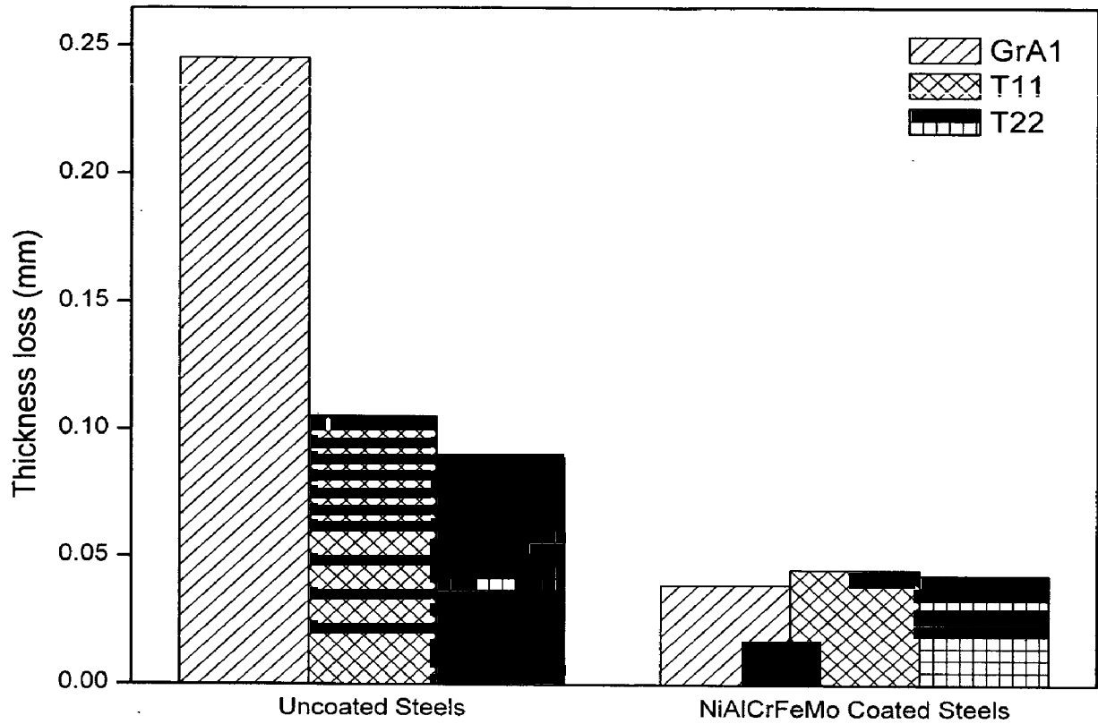
Fig.7.20 Bar chart indicating the thickness lost in mm for the uncoated and NiAlCrFeMo coated steels after 1000 hours of exposure to super heater zone of coal fired boiler.
