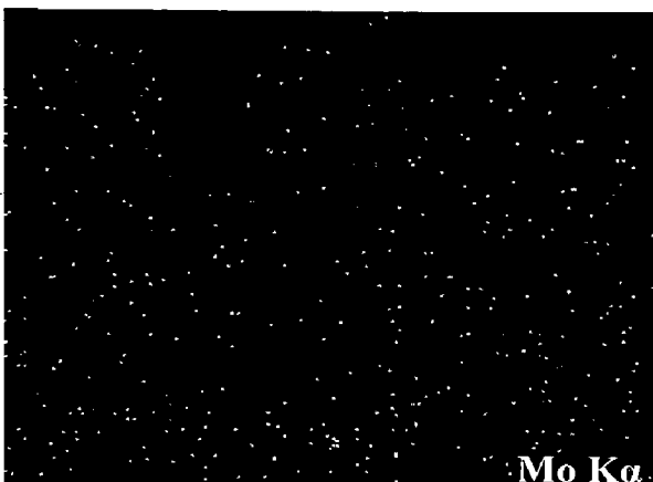
Fig.6.34 BSEI and elemental X-ray mapping along the cross-section of the NiCrAl coated T22 steels subjected to hot corrosion for 50 cycles in \text{Na}_2\text{SO}_4 - 60\%\text{V}_2\text{O}_5 environment at 900^\circ\text{C}
