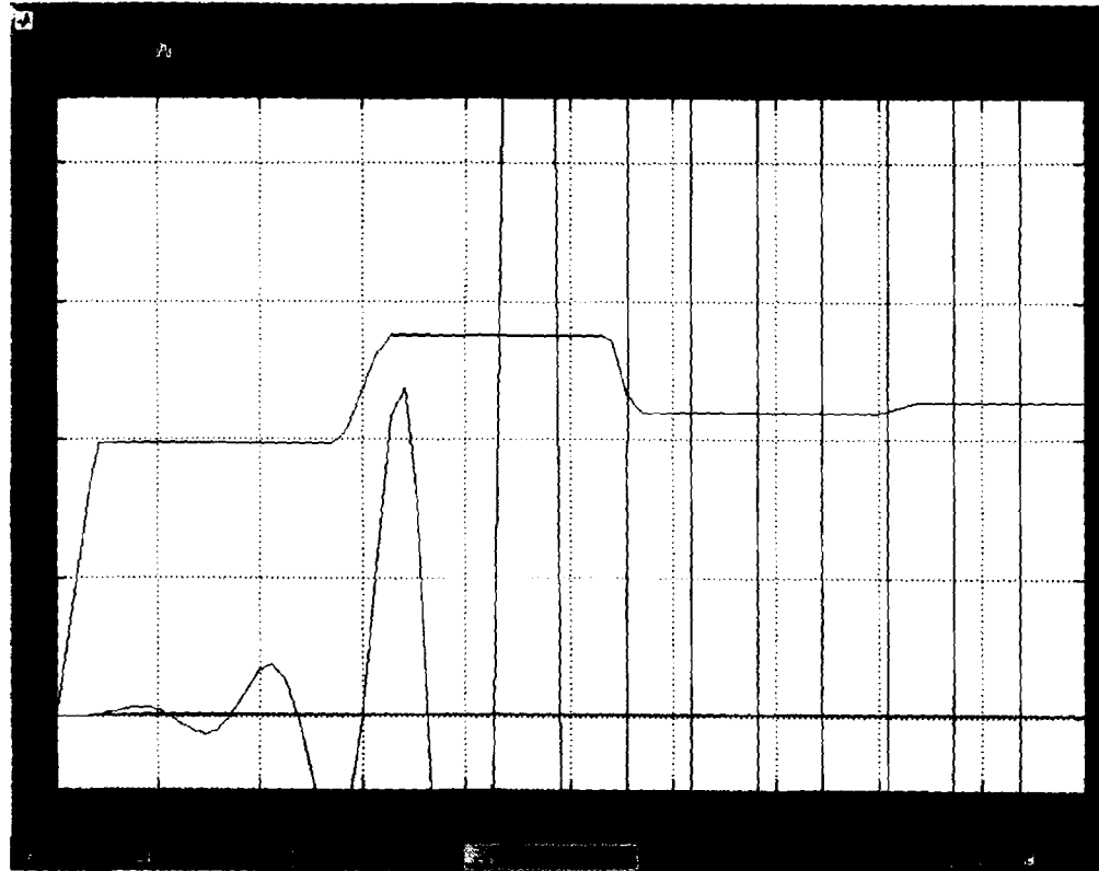
Figure 3.34 Output for varying input- servo model for the basis weight when the value of K_i is 0.001
