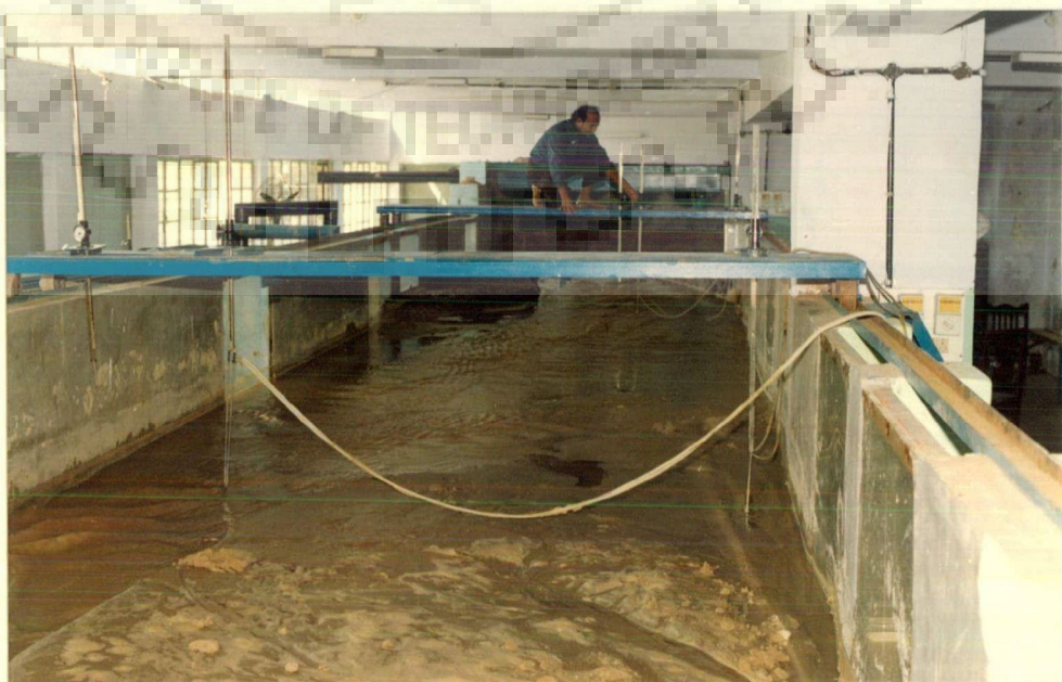
Plate A2.2c: BRAIDING CONDITION WITH MULTIPLE CHANNEL OF RUN - 10 AFTER 20 HOURS OF RUNNING
