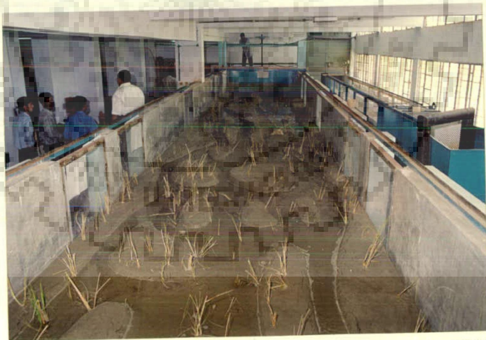
Plate 3.6b: SIMULATED PLAN FORM OF MODEL STUDIES OF THE BRAHMAPUTRA RIVER IN RUNNING CONDITON
