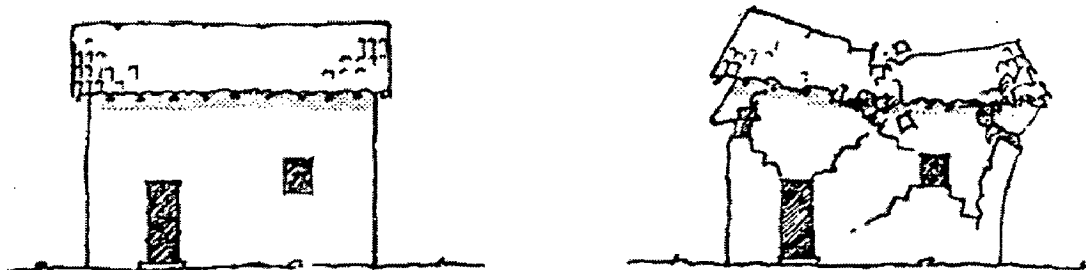
Figure 5.3 Failure in mud walls
