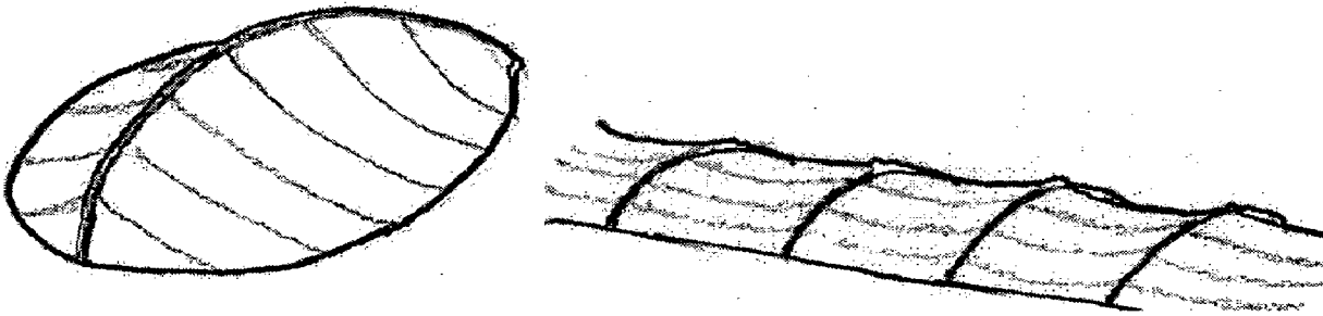
Fig 4.6 Central Arch Supported Form
