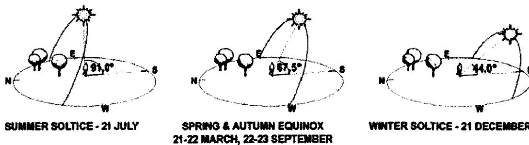
Figure 4.4 Illustrates sun paths as a means for predicting shaded areas.
