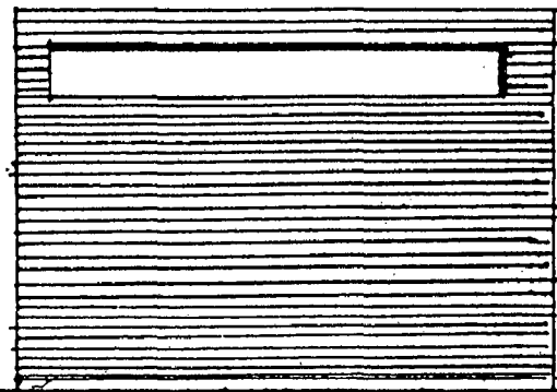
Fig101. High windows are more secure
