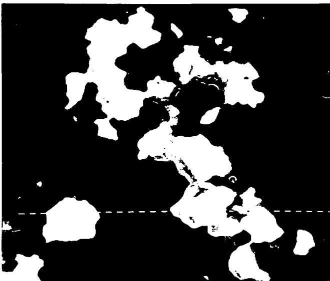
FIG.4.4 SEM pictures of polished specimen, showing typical characteristics of gravity chill cast composites. (a) and (b) SEM pictures of polished specimens showing MgO coating around Al_2O_3 particle. Note that part of the coating has been erased during polishing. Also, the coating can be seen to be intact on comparatively smaller Al_2O_3 particle, (c) picture shows coagulation of Al_2O_3 particles forming a chain-like structure, (d) SEM picture showing the presence of micro voids at particle/matrix interface.
