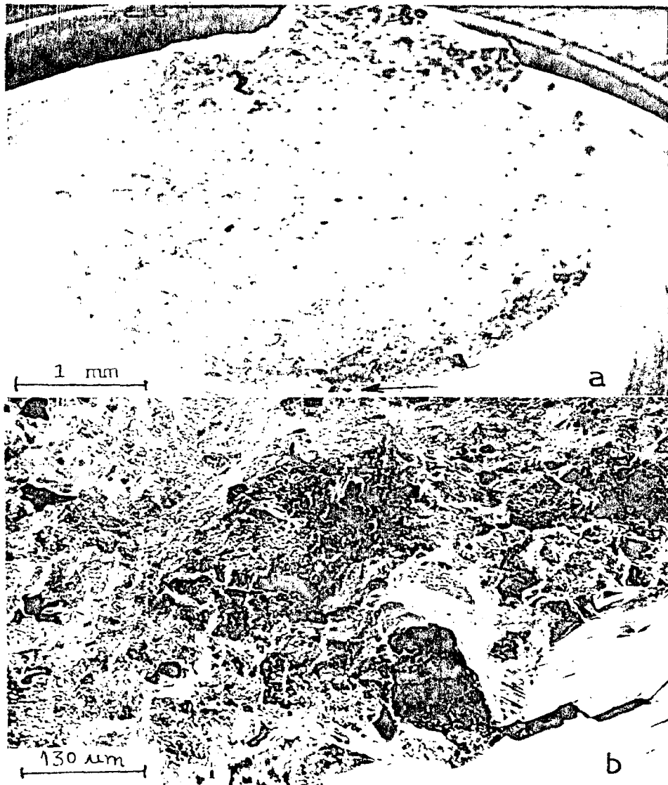
5.17 Microstructure of the 1033 K tensile tested BH3 specimen showing the propagation of cracks along the boride films.
