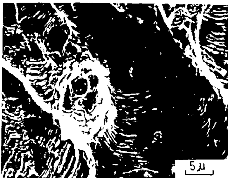
FIG. 4.27 STRAIGHT PARALLEL AND REGULARLY SPACED STRIATIONS IN FATIGUE TESTED AS QUENCHED SAMPLE.
