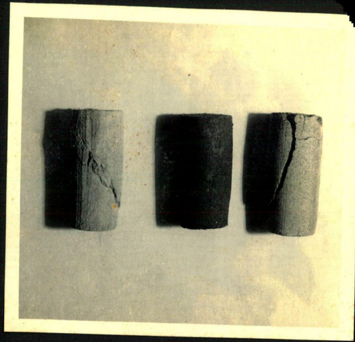
8. TYPICAL MODES OF FAILURE
