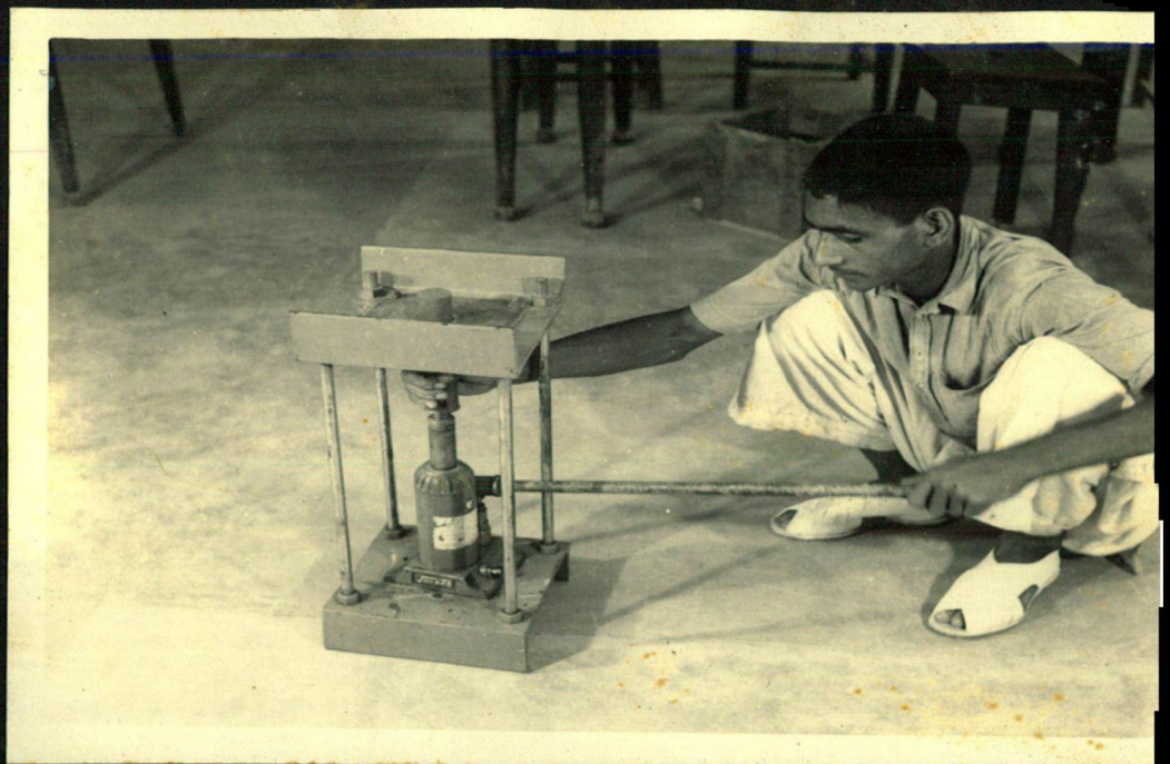
5. EXTRUDING TRIAXIAL SAMPLE FROM CUTTER
