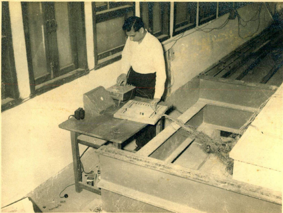
23.5. Measurement of deflections and strains a) Dial gauges in position, b) Reading SR 1 strain Indicator
