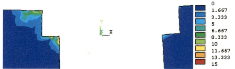
(b 1 ) Principal Stress S1 at brackets ( E=E_c/10 )
