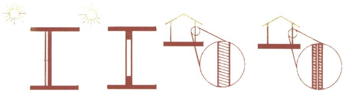
Figure 2.4.4.1.13 Thick walls and cavity walls help in storing heat and create time lag (Source: A Krishnan et al)
