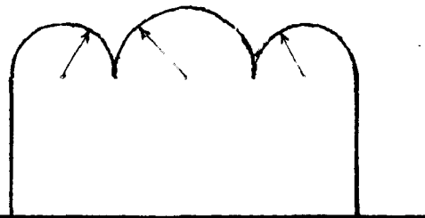
THE RADIUS OF CURVATURE OF CEILING SURFACES SHOULD BE LESS THAN HALF THE HEIGHT OF CEILING.
