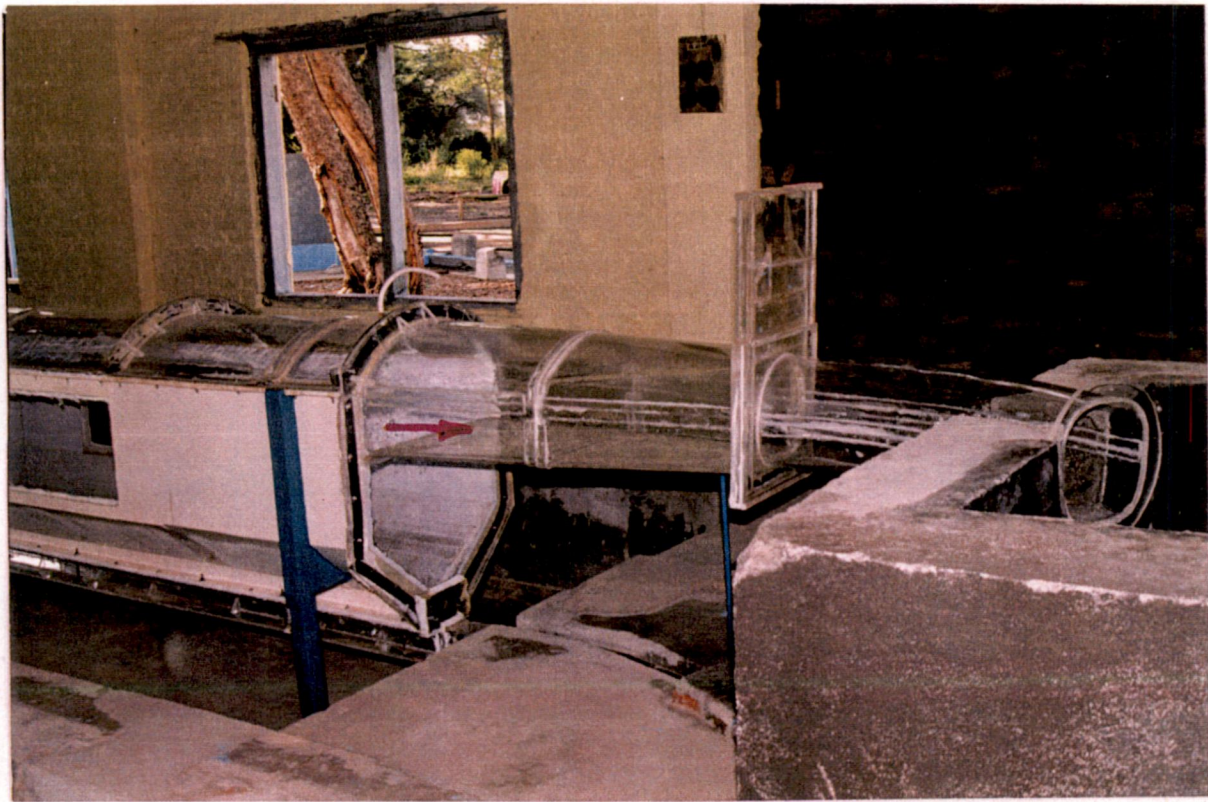
Photo No. 3 : Outlet Transition
