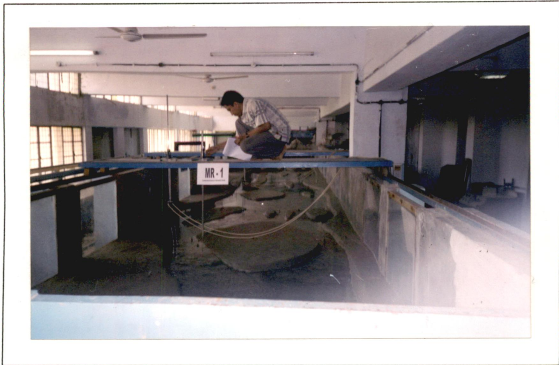
Measuring water surface level using pointer gauge
