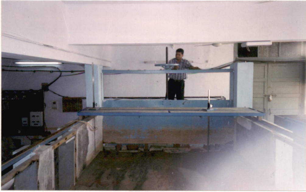
Control gate fixed at down stream of the flume
