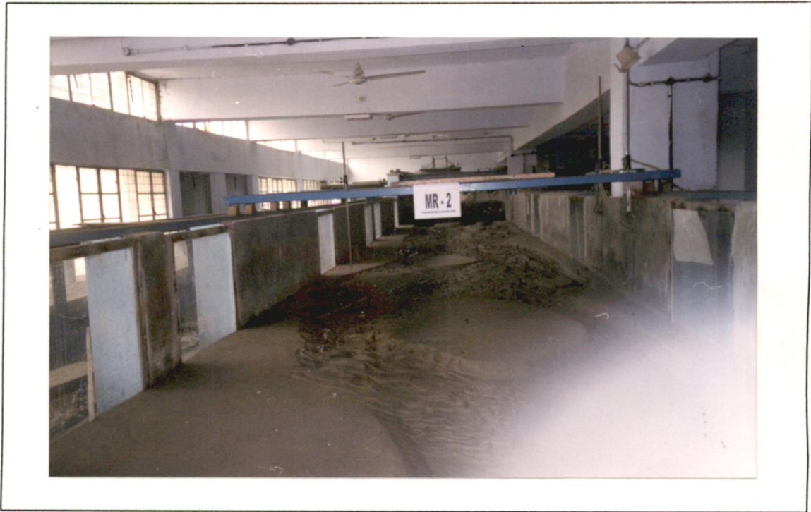
Bed form pattern at the end of experiment Run - 2
