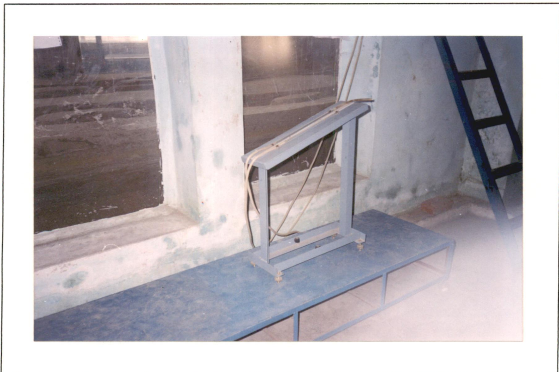
Photograph showing manometer of the pitot tube
