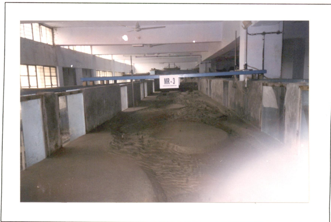
Bed form pattern at the end of experiment Run - 3
