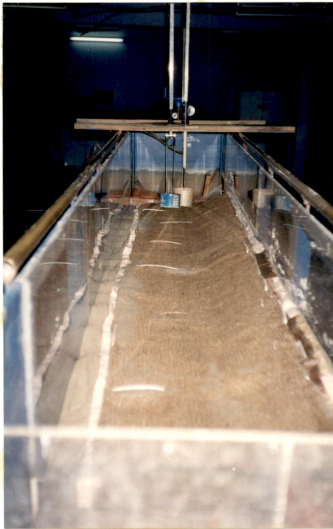
Untreated jute type I (weight 732GM/M 2 ) laid on the flume bed and bank as the covered layer.
