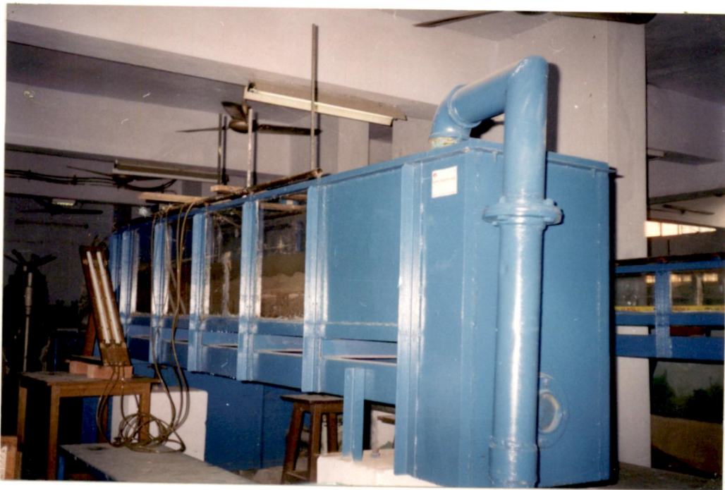
Side view of experimental set-up. Spindle of the fixed screw fixed on the masonry pillar.
