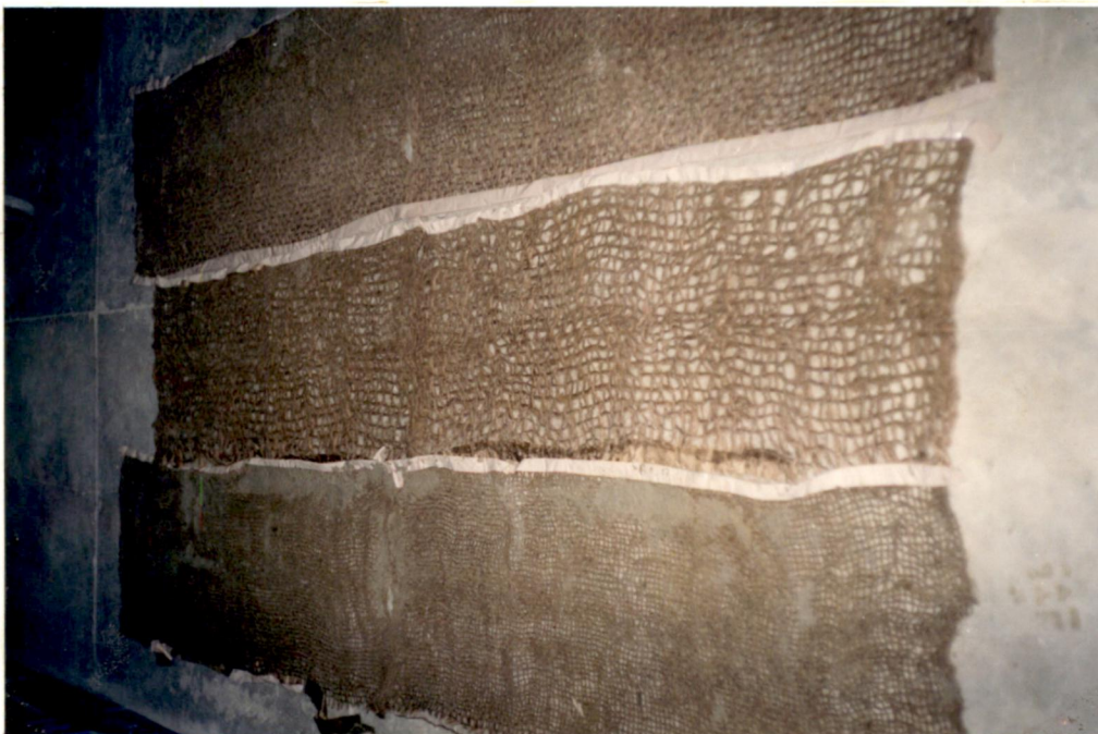
Untreated jute of different type used for bed and bank preparation as a covered layer.
