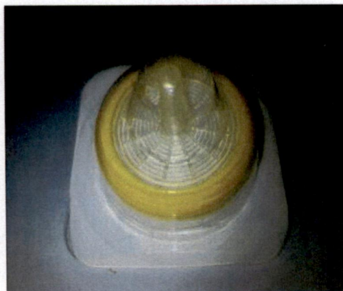
Figure4.2-Showing the 0.45 micron filter
