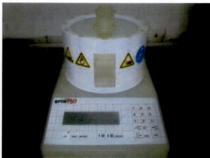
Figure4.4- showing the spin coating machine used.
