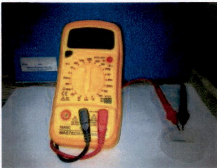
Figure 4.3 -showing the testing of the FTO glass substrate
