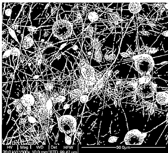
Trial: 3 , PEO: PCL proportion: 1:1, Chloroform: acetic acid proportion: 20:80, Voltage: 18 kV, Flow rate: 0.3 ml/hr Fiber diameter: 249.78 \pm 54 nm
