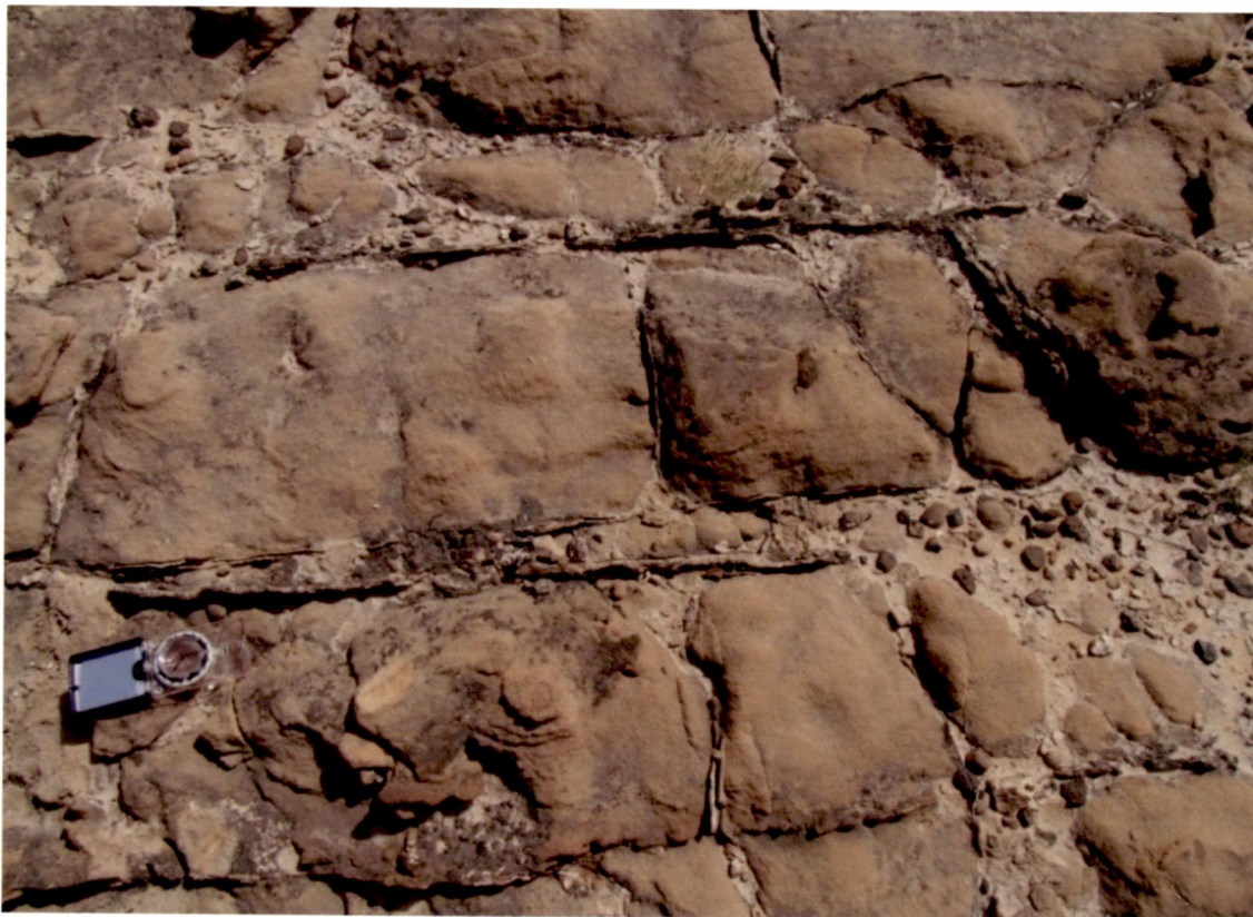
Figure 3.6 Two orthogonal sets of deformation bands giving rectangular zones of undeformed areas.
